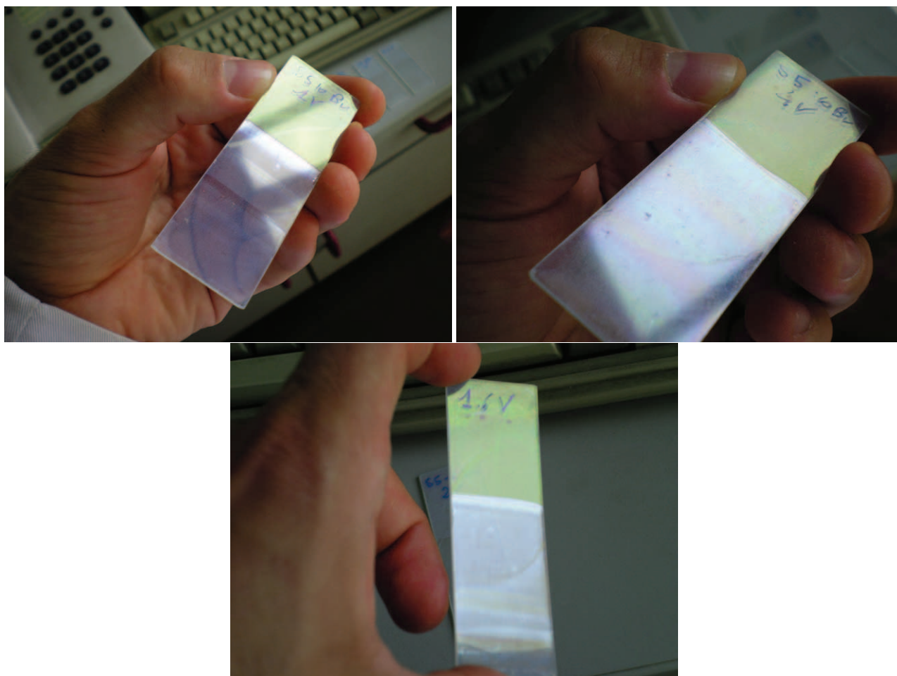
Figure S1: Pictures of colloidal crystals made of PS batch #2 obtained with spin-coating. The upper part of the films is the PS colloidal crystal not infiltrated with TiO 2 showing a green colour due to the second order Bragg diffraction. The lower portion of the film has been infiltrated with TiO 2 with the dip-coating technique showing a blue-violet colour due to the change of the effective refractive index of the film, because of the replacement of air with TiO 2
