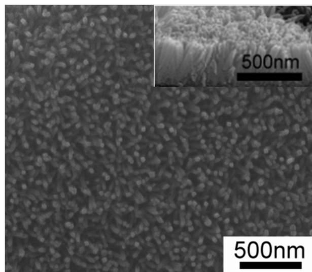
Fig. S3: The SEM image of the rutile nanowire arrays grown in the vapor of 6.0 M HCl solution at 140 °C for 3.0 h.
