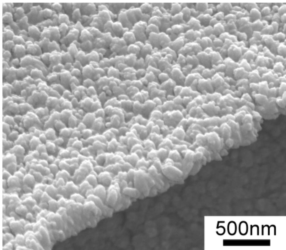
Fig. S1: The SEM image of the rutile nanowire arrays grown with 6.0 M HCl solution at 100 °C for 6.0 h.
