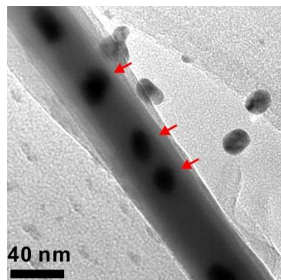
**Fig. S3** High resolution transmission electron microscopy (TEM) images for the Au NPs embedded in the NPW. A 200kV field emission TEM (Tecnai F-20) was used for the TEM imaging. The dark spots (red arrows) represent the embedded Au NPs in the NPW.
