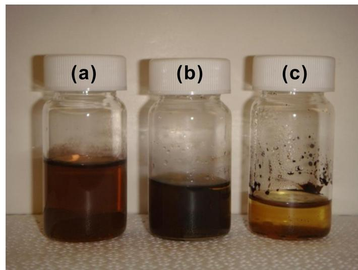
**Fig. S1** Continuing development of the PANI and Au composite nanostructures. (a) PANI and Au NP solution without light curing. Reddish color in water phase indicates the formation of Au NP chains. (b) PANI and Au NP solution after a process of polymer curing (5 min, tungsten halogen lamp). The purple greenish color indicates the oxidized states of PANI. (c) PANI and Au NP aqueous solution of (b) after 1 week. Greenish water phase was still visible after precipitation of heavy aggregates.
