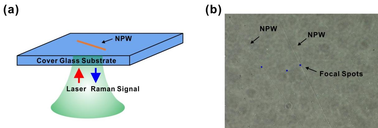
**Fig. S5** Raman spectroscopy for NPWs. (a) Schematic diagram showing a micro-Raman microscope equipped with an inverted optical microscope (Axiovert 200, Zeiss). A 300 W He-Ne laser (Melles Griot) with the excitation wavelength of 632.8 nm was used as the excitation source. The laser was focused on a NPW on a cover glass slip. The Raman spectra of the sample were recorded in the range of  $500 \sim 2,000 \text{ cm}^{-1}$ . (b) Optical microscopy image of NPWs and the focal spots.
