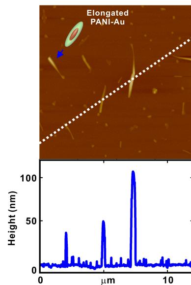
**Fig. S2** Tapping-mode AFM topography image (top) and the height profile (bottom) of the elongated PANI-Au nanoseeds. The heights of the elongated PANI-Au nanoseeds varied in the range from a few nm to 100 nm.
