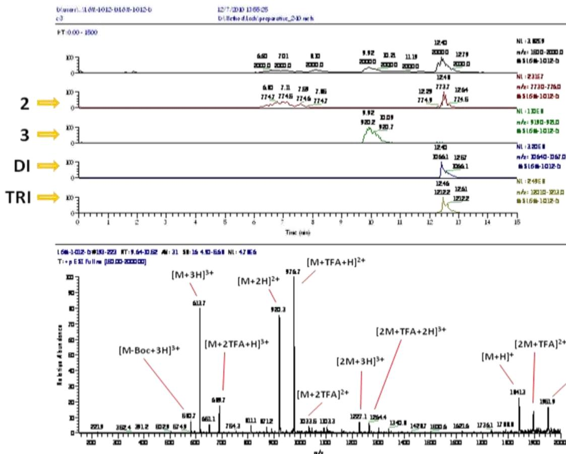
**Supporting Figure 1.** Preparative MS chromatogram (Alltima HP C18, 5  $\mu$ M, 125 mm length, ID 20 mm) of **3** during purification. Above: Total Ion Count and masses corresponding to non-functionalized (**2**), mono-functionalized (**3**), and di- and tri-functionalized cysteamine-cyclodextrin (DI, TRI). Below: mass spectrum of the product peak 9.64-10.52 min.
