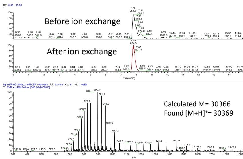
**Supporting Figure 9.** Top: LC/MS spectra of mYCDNH<sub>2</sub> before and after ion exchange chromatography (TIC signal); Bottom: MS spectrum of the purified protein after ion exchange with its deconvoluted mass.
