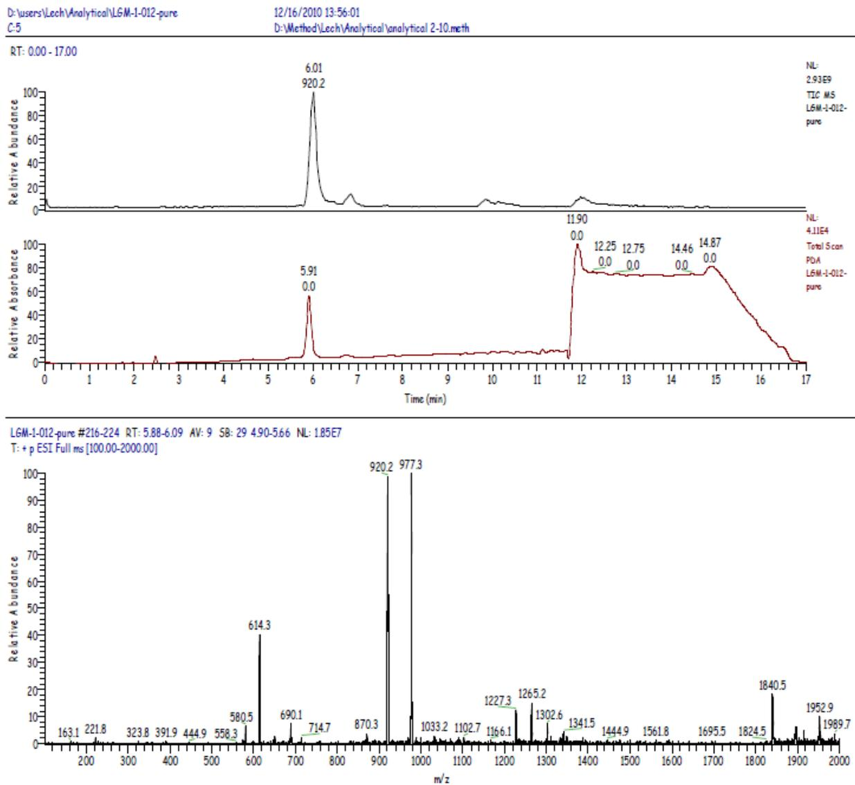
**Supporting Figure 2.** Analytical LC-MS spectrum (Alltima HP C18, 5  $\mu$ M, 125 mm length, ID 2 mm) of **3** after purification. Above: TIC (top) and UV (bottom) after purification; Below: mass trace of the product peak 5.88-6.09 min.
