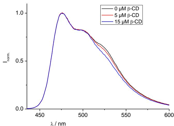
**Supporting Figure 10.** Fluorescence emission spectra of 0.5  $\mu\text{M}$  protein complex mYCD-mCLA (black) after addition of 5  $\mu\text{M}$  (red) and 15  $\mu\text{M}$   $\beta$ -Cyclodextrin.
