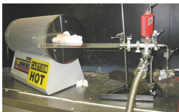
**Figure S1.** Actual pictures of the safe and simple experimental setup that is used in the synthesis of graphene films on copper foil.
