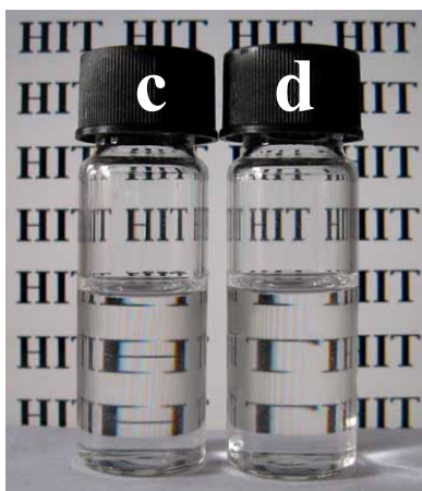
Figure S7. Fourier transform infrared (FT-IR) spectra of BaYF 5 nanocrystals before (a) and after (b) ligand exchange using PAA. Photographs of colloidal solutions of the BaYF 5 nanocrystals (50-60nm) dispersed in cyclohexane and water before (c) and after (d) PAA modification. The FT-IR spectra were used to characterize the functional groups present on the surface of nanocrystals. The band at 1374 cm -1 characterizing the mode of the C=O (N-CO-OH) stretching vibration in the EDTA molecule became weaker after ligand exchange (Figure S7b), suggesting the decreased EDTA molecule on the surface of BaYF 5 nanoparticles. Moreover, the bands at 1738 cm -1 and 2945 cm -1 newly appeared in Figure S7b characterize the -COOH group and the stretching vibration of methylene (CH 2 ) in the long alkyl chain, respectively, illustrating the presence of the PAA molecule on the surface of BaYF 5 nanoparticles. These observations give a strong evidence of the successful exchange of EDTA by the ligand of PAA. The broad band between 2800 cm -1 and 3600 cm -1 arises from the O-H stretching vibration (COO-H).
