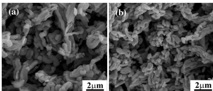
**Fig. S2** SEM images of CMK3 and CMK3-S composites. (a) As-synthesized CMK3; (b) CMK3-56 (56 wt.% sulfur loading) after wet impregnation with sulfur-CS<sub>2</sub> solution and 155 °C annealing.
