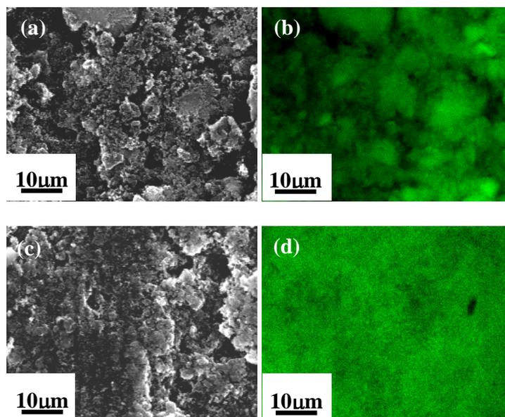
**Fig. S6** SEM images and S elemental mapping results of the MC22-50-Clevios P electrode before and after cycling. (a) SEM image of the MC22-50-Clevios P electrode before cycling. (b) S elemental mapping of the MC22-50-Clevios P electrode before cycling. (c) SEM image of the MC22-50-Clevios P electrode after 100 cycles. (d) S elemental mapping of the MC22-50-Clevios P electrode after 100 cycles.
