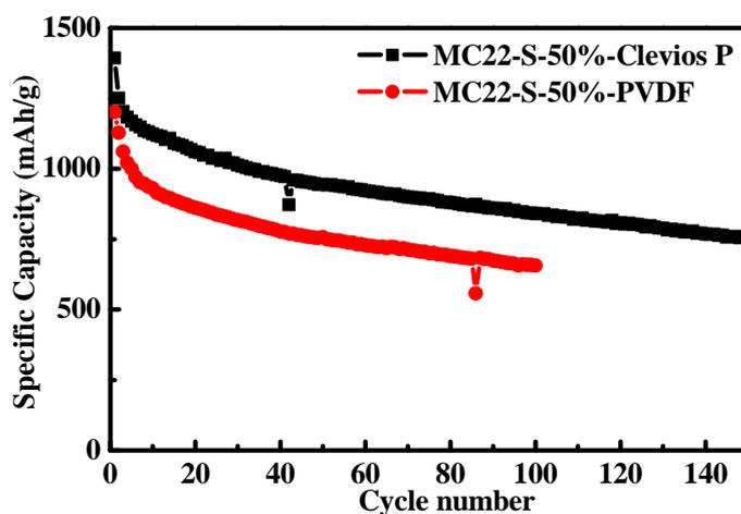
**Fig. S5** Long term cycle stability of MC22-50 composite electrodes using Clevios P and PVDF, respectively, as binders.
