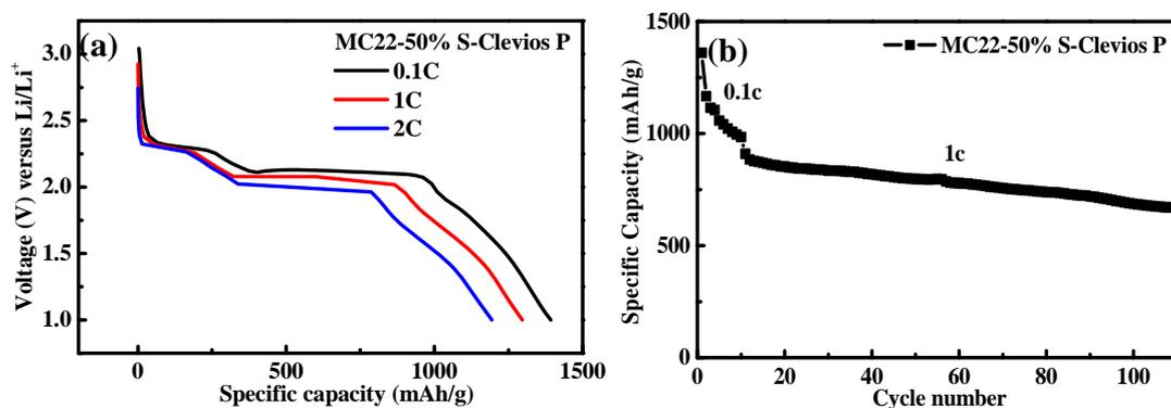
**Fig. S7** Rate performance of MC22-50-Clevios P electrodes. a) First cycle discharge curves of MC22-50-Clevios P electrodes at different current densities of 168 mA/g (0.1C), 1680 mA/g (1C), and 3340 mA/g (2C) respectively. b) Long term cycling of a MC22-50-Clevios P electrode after a 110 cycle test under different charge-discharge current densities of 168 mA/g (0.1C) and 1680 mA/g (1C) respectively.
