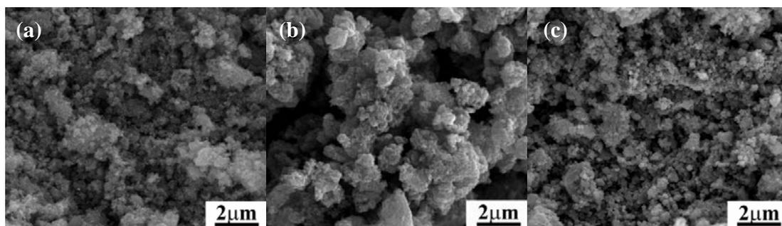
**Fig. S1** SEM images of MC22 and MC22-S composites. (a) As-synthesized MC22; (b) MC22-83 (83 wt.% sulfur loading) after wet impregnation with sulfur-CS<sub>2</sub> solution and 155 °C annealing; (c) MC22-50 (50 wt.% sulfur loading) after wet impregnation with sulfur-CS<sub>2</sub> solution and 155 °C annealing.
