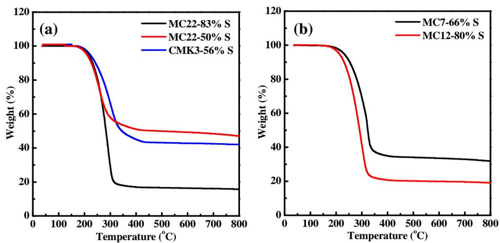
**Fig. S3** TGA curves of MCS composites recorded under nitrogen with a heating rate of 10 °C/min.
