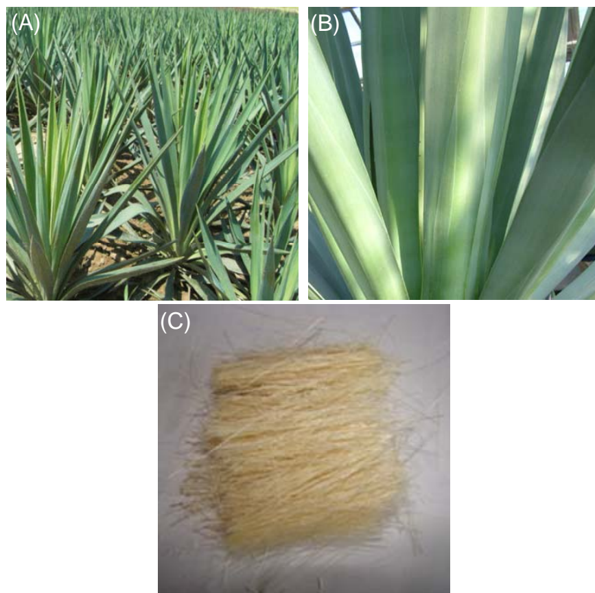
Fig. S1 Photographs of (A) natural sisal in a plantation (B) leaves of sisal plant (C) sisal fibers. Sisal fibers are obtained by extraction from the shredded leaf tissues of sisal.
