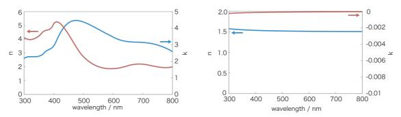
S2. Real and imaginary parts of refractive indices of Os (left) and PB (right) measured by using a spectroscopic ellipsometry, respectively.
