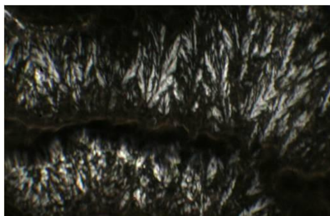
Figure S3. Birefringent texture for a hexagonal phase mixture consisting of 55% \text{PEO}_{37}\text{PPO}_{58}\text{PEO}_{37} , 40% formamide and 5% heptane under ambient conditions.
