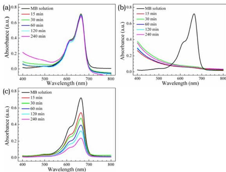
**Fig. S3** UV-Vis spectra of the original and treated with (a)  $\text{Mg}(\text{OH})_2$ , (b) GO, (c) rGO (100 mg) organic dyes solutions ( $\text{MB}$ ,  $2.0 \times 10^{-5}$  M, 50 ml) for various times.
