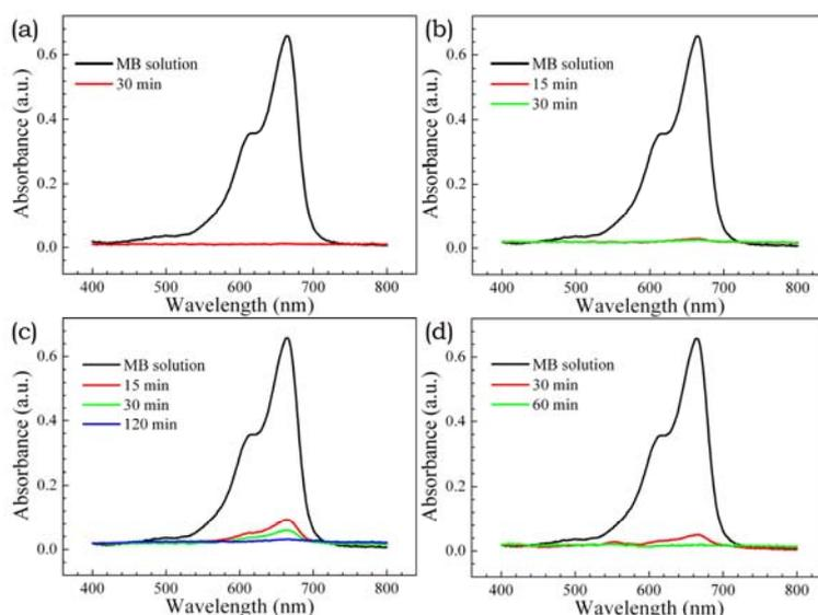
**Fig. S2** UV–Vis spectra of the original and treated with MGC (100 mg) organic dyes solutions (MB,  $2.0 \times 10^{-5}$  M, 50 ml) for various times, and in various cycles. (a) 1st, (b) 2nd, (c) 3rd, and (d) 4th cycle.
