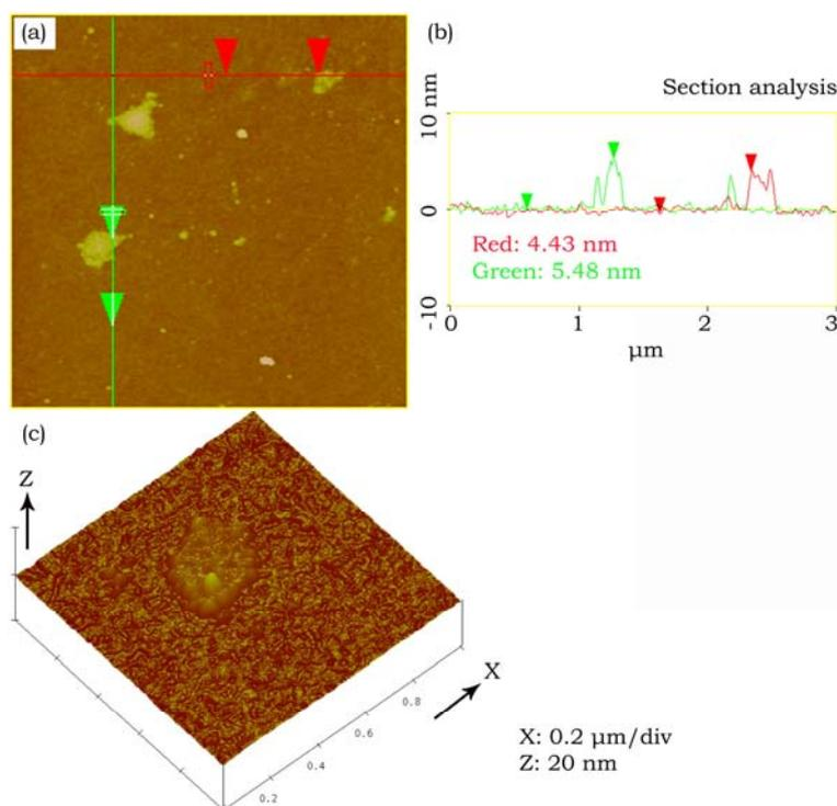
Fig. S1 (a) Typical AFM images, and (b) its cross section analysis (c) three dimensional AFM images of MGC.
