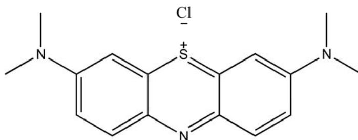
**Fig. S4** The molecule structure of MB.
