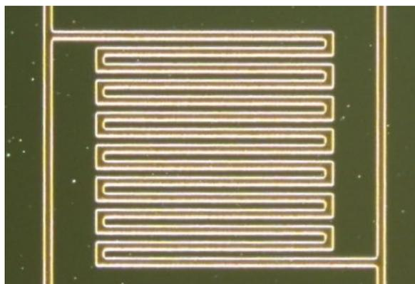
**Figure S1.** A serpentine type microheater of Au fabricated on a Si substrate for electrophoretic deposition of PCDA vesicles.
