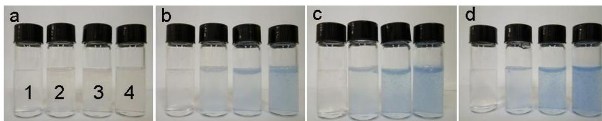
**Figure S2.** Radical induced polymerization of PCDA-EDEA 2 vesicle solutions using potassium peroxydisulfate (KPS). 1- Control (pure PCDA-EDEA) 2- 15 $\mu$ L: 3mL PCDA-EDEA 3- 30 $\mu$ L KPS: 3mL PCDA-EDEA 4- 60 $\mu$ L KPS: 3mL PCDA. (a) right after mixing the solutions (b) after 30 min (c) after 1 hr and 30 min (d) after 24 hr.
