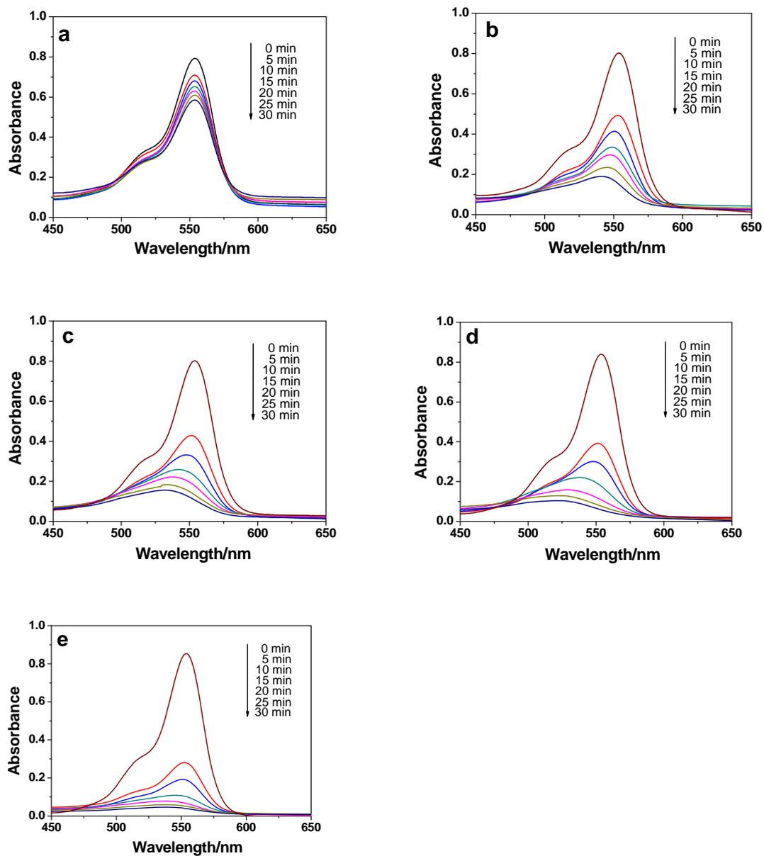
**Figure S1.** The absorption spectra of the RhB solutions at different exposure times in the presence of different samples a) S0, b) S5, c) S10, d) S15 and e) S20.
