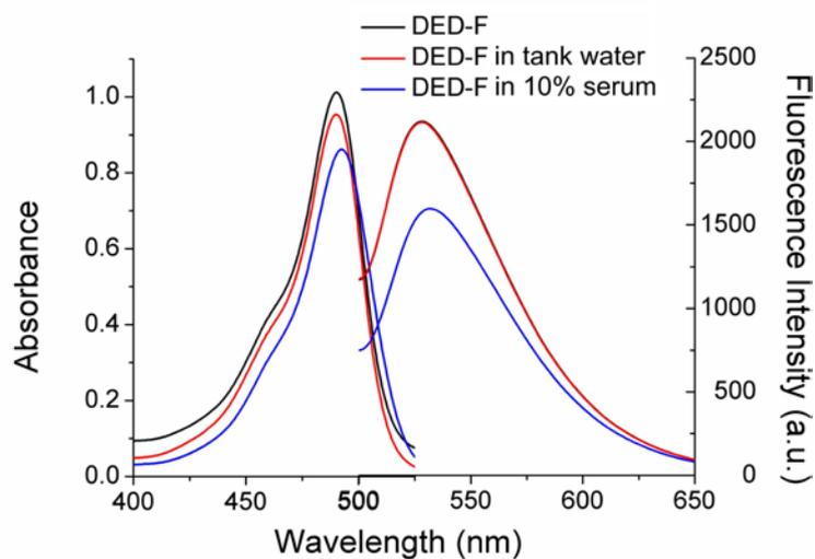
**Figure S3** The absorption and emission spectra of 150  $\mu\text{g/mL}$  DED-F NPs in PBS, regular tank water and 10% serum at room temperature.
