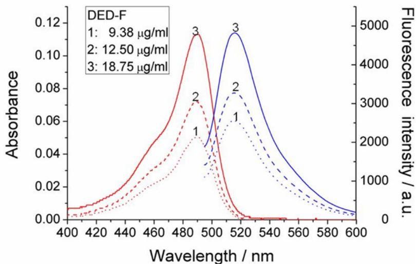
**Figure S2** The absorption and emission spectra of DED-F NPs in PBS with different concentrations: (1) 9.38  $\mu\text{g/mL}$ ; (2) 12.5  $\mu\text{g/mL}$ ; (3) 18.75  $\mu\text{g/mL}$ .
