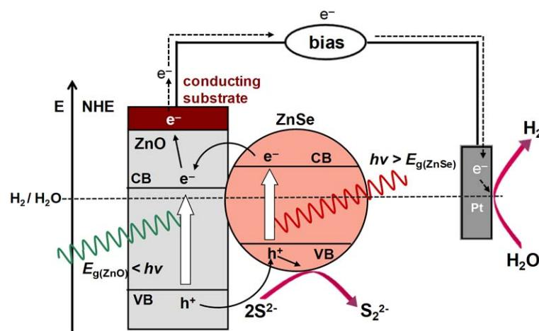
**Figure S1.** Schematic diagram showing the energy band structures of a ZnO/ZnSe heterostructure in photoelectrochemical water splitting.
