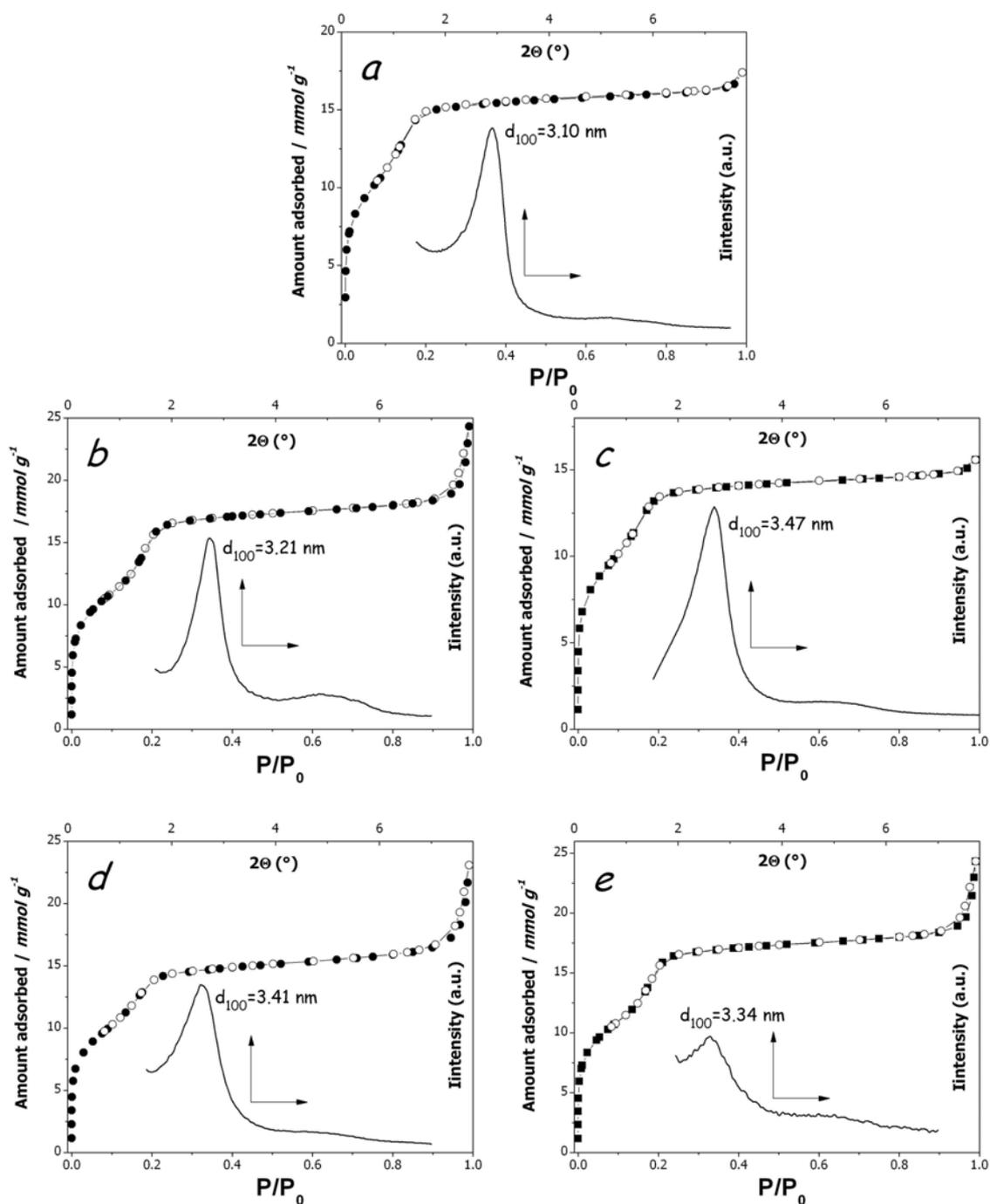
**Figure I.** Nitrogen adsorption (●) and desorption (○) isotherms at 77 K for the MSS type materials studied: a) purely siliceous MSS, b) Al-MSS-44, c) Al-MSS-22, d) Al-MSS-11, e) Al-MSS-7. The insets show the XRD patterns for the five samples.
