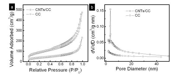
Figure S1 (a) Nitrogen adsorption/desorption isotherms of sample. (b) The pore size distribution plots that were calculated by the BJH formula in the adsorption branch isotherm.
