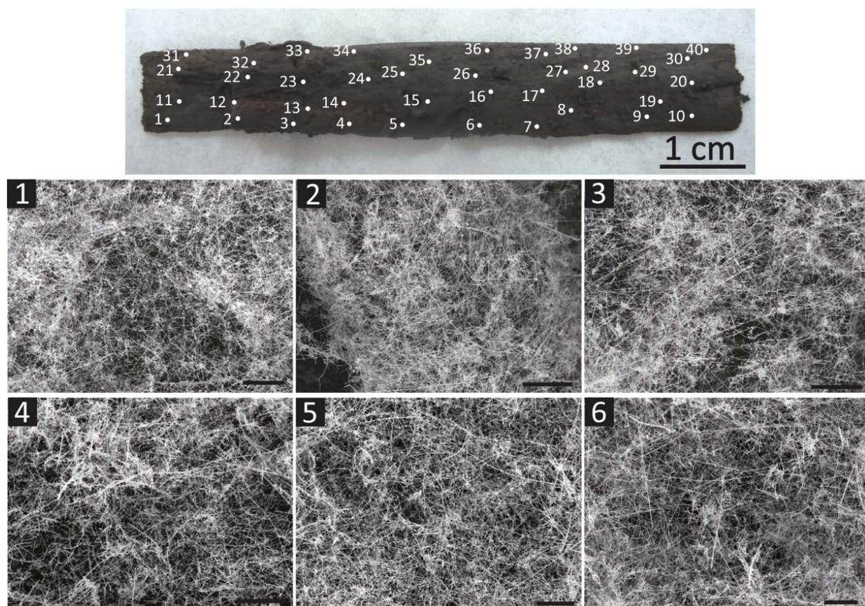
**Fig. S2-1** Photograph of Ge nanowires on silicon substrate and marked out 40 points randomly-picked regions and SEM image of LICVD-grown Ge NWs synthesized from DPG with three-times injection of 40 different randomly-picked regions. Six regions of the 40 points randomly-picked SEM image, corresponds to the region 1 to the region 6. Scale bar, 50 μm.
