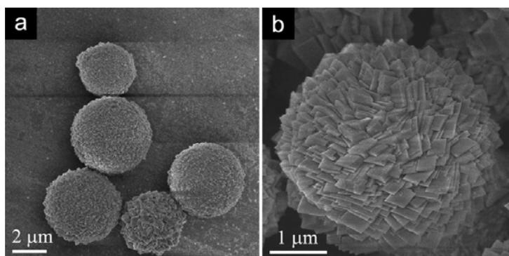
**Figure S2.** FESEM images of ZnCO<sub>3</sub>-MnCO<sub>3</sub> composite microspheres.
