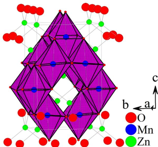
**Figure S4.** Schematic crystal structure of ZnMn<sub>2</sub>O<sub>4</sub> spinel.
