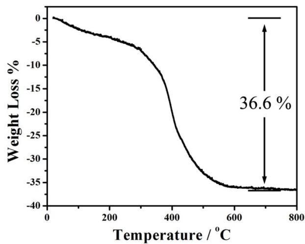
**Figure S3.** TGA curve of the ZnCO<sub>3</sub>-MnCO<sub>3</sub> composite under air flow with a temperature ramp of 10 °C min<sup>-1</sup>.
