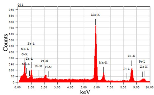
**Figure S5.** EDX spectrum of the ZnMn<sub>2</sub>O<sub>4</sub> hollow microspheres.
