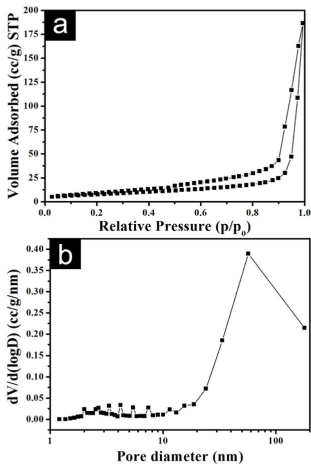
**Figure S6.** N<sub>2</sub> adsorption-desorption isotherm (a) and pore size distribution (b) of the ZnMn<sub>2</sub>O<sub>4</sub> hollow microspheres.
