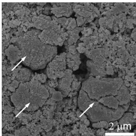
**Figure S7.** FESEM images of the electrode made of  $\text{ZnMn}_2\text{O}_4$  hollow spheres after 100 cycles at  $400 \text{ mA g}^{-1}$ .
