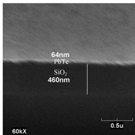
Figure S6. SEM image of the PbTe NC thin film thickness assembled at 45 °C for 12 h
