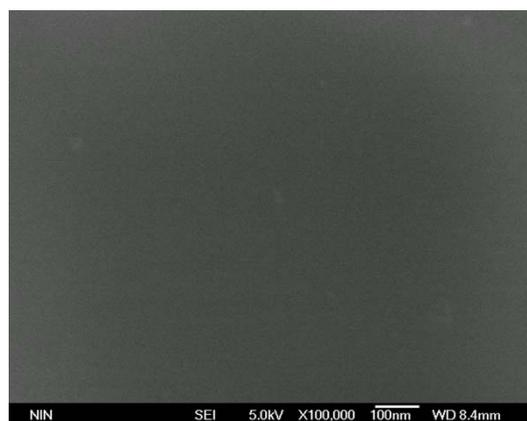
Figure S4. SEM image of the PbTe NC thin film assembled at 45 °C for 2 h
