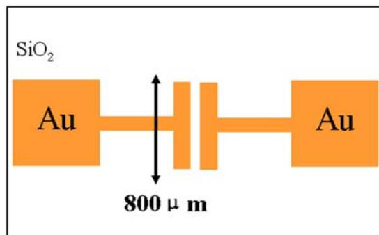
Figure S1. Schematic of Si/SiO<sub>2</sub> substrate structure in the experiment. Ti/Au contacts are microfabricated on silicon oxide surface.
