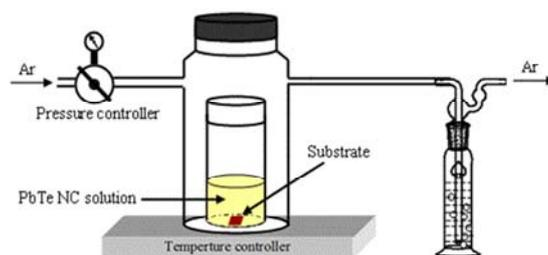
Figure S2. Scheme of the experimental setup for assembling PbTe NC thin films with the NC solution evaporation rate controlled by changing the reaction temperature and velocity of Argon flow.
