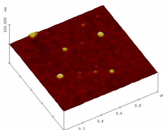
Figure S3. AFM morphology of the PbTe NC thin film on Si/SiO<sub>2</sub> substrates assembled at 45 °C for 2 h
