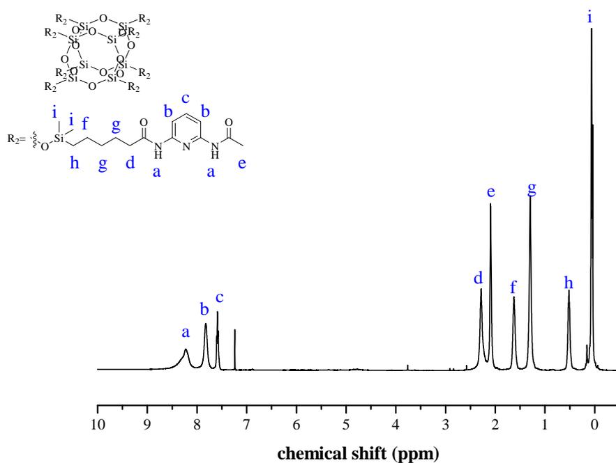
**Figure S17.** <sup>1</sup>H NMR spectra of Octakis[dimethyl(N-(6-acetamidopyridin-2 yl)siloxy] silsesquioxane (ODAP-POSS).
