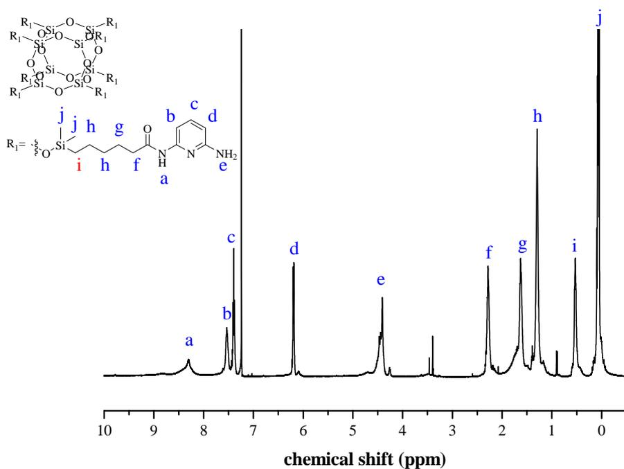
**Figure S15.** <sup>1</sup>H NMR spectra of Octakis[dimethyl(N-(6-aminopyridin-2-yl)siloxy]silsesquioxane.
