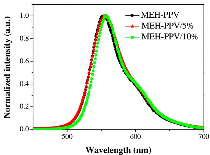
**Figure S7.** EL spectra of MEH-PPV/U-PY/ODAP-POSS (90/10) based device.
