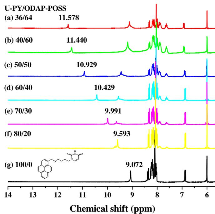
**Figure S1.**  $^1\text{H}$  NMR spectroscopic titration. Amide region of the  $^1\text{H}$  NMR spectrum of U-PY after the addition of ODAP-POSS.
