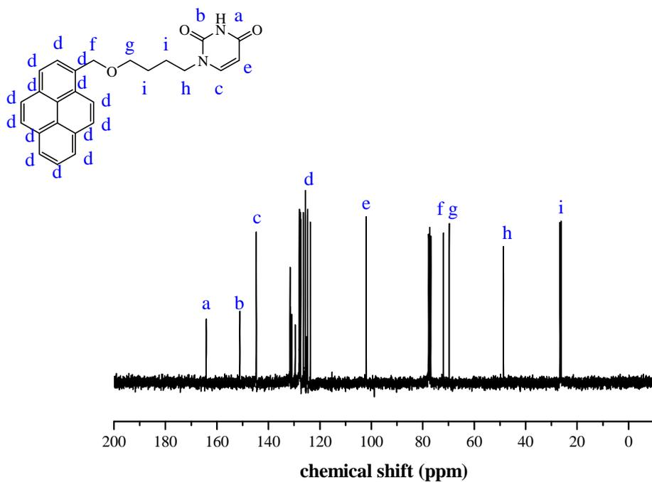
**Figure S12.**  $^{13}\text{C}$  NMR spectra of 4-uracilbutyl-1-methylpyrene ether (U-PY).
