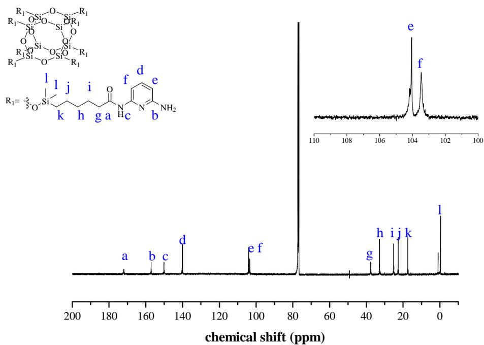
**Figure S16.** <sup>13</sup>C NMR spectra of Octakis[dimethyl(N-(6-aminopyridin-2-yl)siloxy]silsesquioxane.
