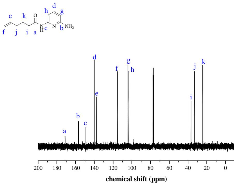
**Figure S14.** <sup>13</sup>C NMR spectra of N-(6-aminopyridin-2-yl)hex-5-enamide.
