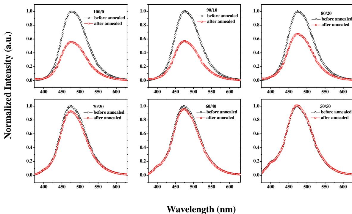
Figure S4. Thermal quenching of U-PY/ODAP-POSS composites in films after annealed at 150°C.
