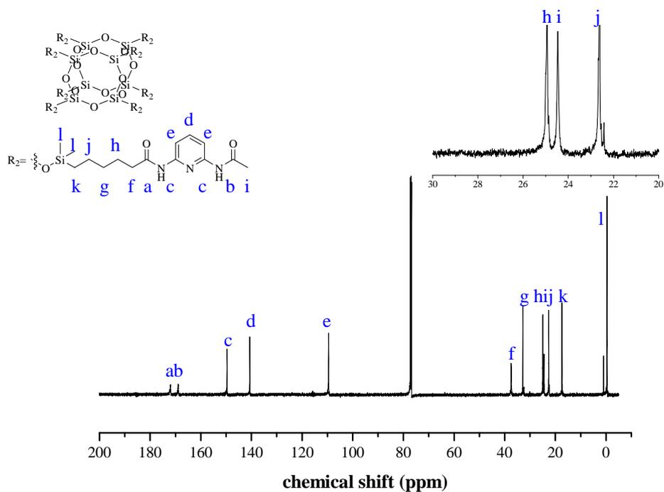
**Figure S18.** <sup>13</sup>C NMR spectra of Octakis[dimethyl(N-(6-acetamidopyridin-2 yl)siloxy] silsesquioxane (ODAP-POSS).
