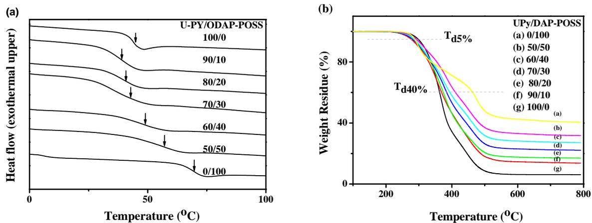
Figure S3. DSC thermograms (a) and TGA thermal degradation patterns (b) for U-PY/ODAP-POSS composites in various weight ratios.
