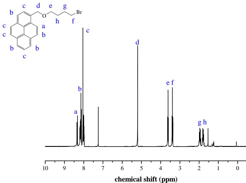
**Figure S9.**  $^1\text{H}$  NMR spectra of 1-((4-bromobutoxy)methyl)pyrene.
