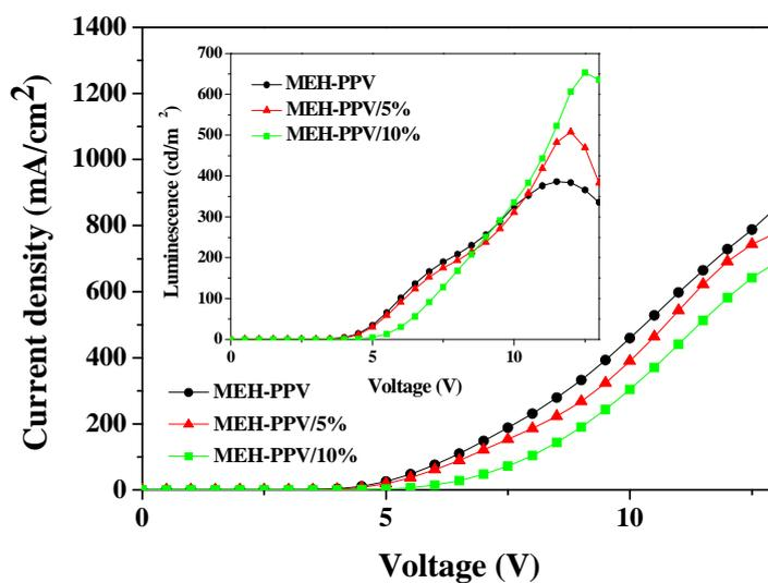
**Figure S6.** Voltage-Current density and Voltage-Luminescence characteristic of MEH-PPV/(U-PY/ODAP-POSS 90/10) based device.
