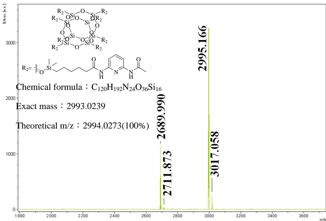
**Figure S8.** MALDI-TOF mass spectrum of ODAP-POSS.
