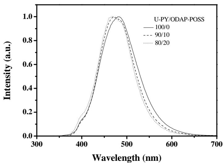
**Figure S5.** Electroluminescence based on the devices ITO/PEDOT:PSS/(U-PY/ODAP-POSS)/TPBI/LiF/Al.
