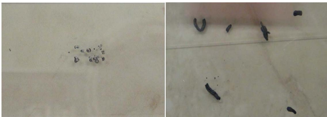
**Fig. S1** Photo images of unexpanded (left) and expanded (right) graphite flakes on glass plate.
