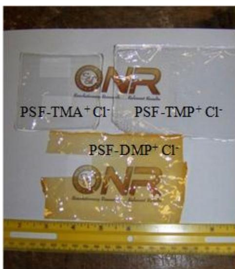
**Fig. S4:** Thin film anion exchange membranes ranging from 40 to 80 μm in thickness.
