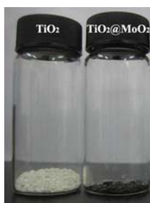
Fig. S1 Digital photos for the powdered samples of the TiO 2 nanofibers (white) and the MoO 2 -modified TiO 2 nanofibers (black).
