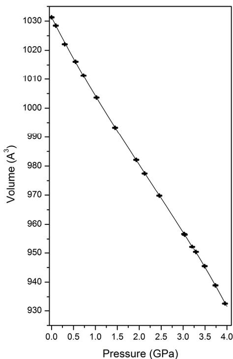
**Figure S1.**  $P$ - $V$  data for **1**. Experimental data points are shown, with error bars, as black circles. The solid black curve represents a 4<sup>th</sup> order BM EoS fit to the data over the 0–4 GPa range ( $w\chi^2 = 0.8$ ).
