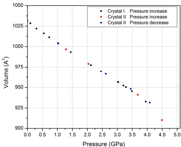
**Figure S2.** Evolution of the unit cell volume of crystals I and II as a function of pressure. Error bars are smaller than the symbols representing the data points.
