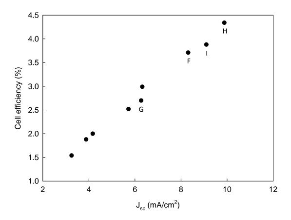
Fig. S1. In general, the cell efficiency increases with the short circuit current density. Selected cell IDs are given.
