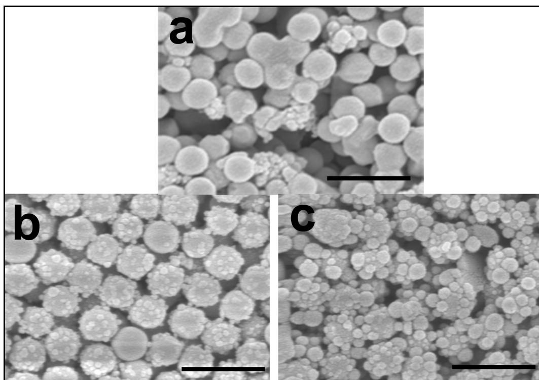
**Figure S2.** SEM images of the particulate film composed of (a) the core-shell  $\text{SiO}_2/\text{PS}$  hybrid particles, (b) Sample A and (c) Sample E. All scale bars are 500nm.
