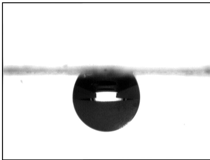
**Figure S1.** Shape of water on the superhydrophobic  $\text{SiO}_2/\text{PS}$  particulate film surface upside down.
