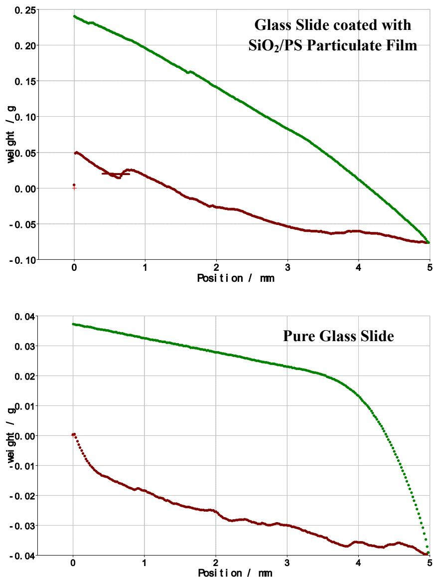
**Figure S3.** Force-position curves recorded when the glass slide was immersed into (Red curves) and pulled out of water (Green curves).
