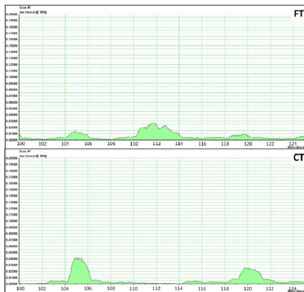
Figure S3 2-D TGA-MASS diagram of FT and CT regarding the ion current corresponding to m/z at 250 and 350 °C, respectively. ( m/z = 100 to 125)
