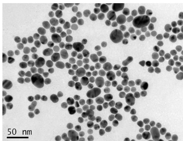
**Fig. S3** TEM images of Au NPs with the average diameter of 20 nm.
