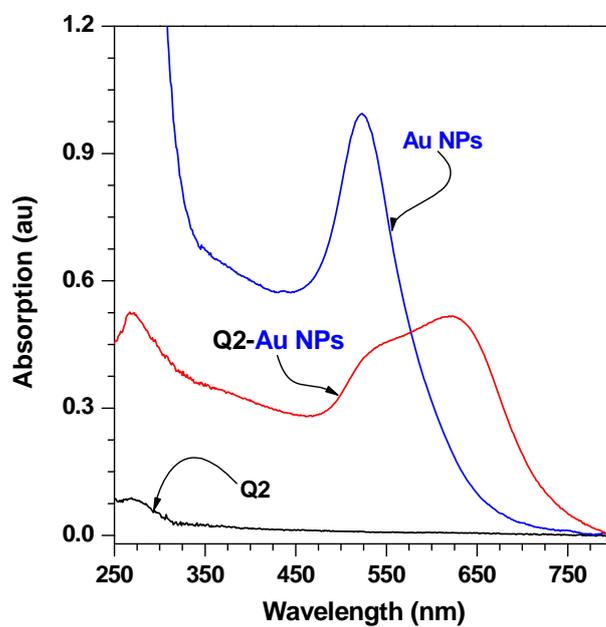
**Fig. S7** Absorption spectra of Q2, Au NPs and Q2-Au NPs in C<sub>2</sub>H<sub>5</sub>OH.
