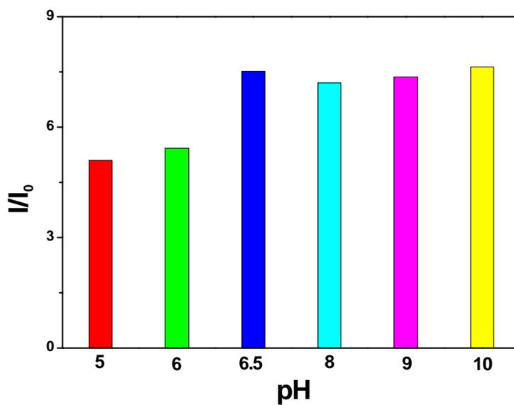
**Fig. S9** The fluorescence response of the Q2-Au NPs to CN<sup>-</sup> at different pH values.
