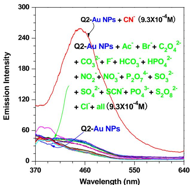
**Fig. S5** Fluorescence Emission spectra of **Q2**-Au NPs in C<sub>2</sub>H<sub>5</sub>OH in the presence of different anions(9.3×10<sup>-4</sup> mol/L). The concentration of **Q2** was 35×10<sup>-6</sup> mol/L and Au NPs was 27.8×10<sup>-5</sup> mol/L. Excitation wavelength (nm): 355.
