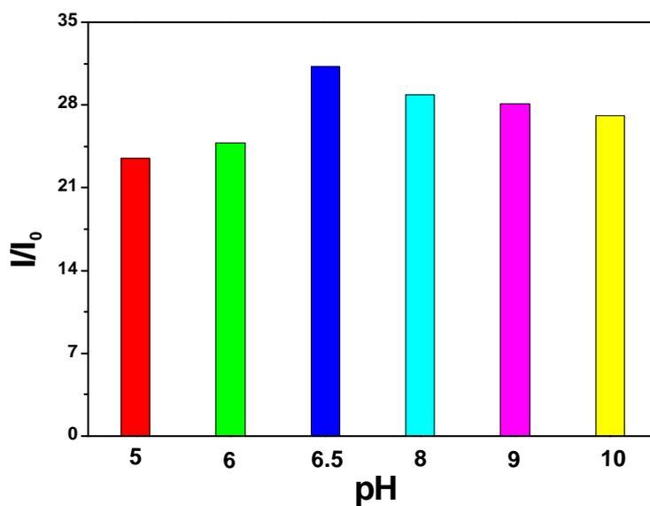
**Fig. S8** The fluorescence response of the Q1-Au NPs to CN<sup>-</sup> at different pH values.
