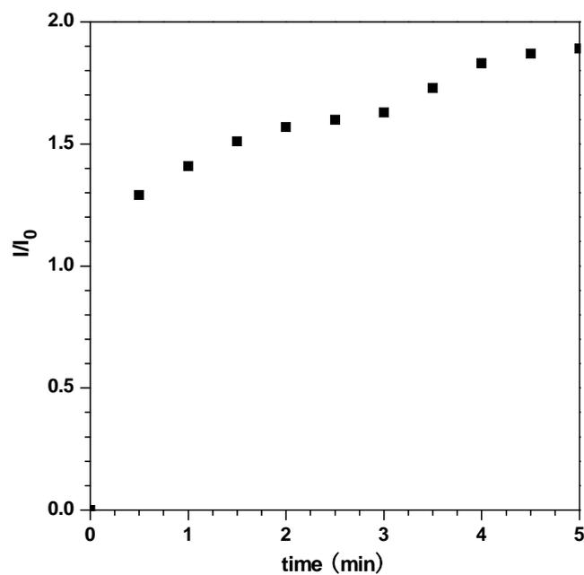
**Fig. S2** Time-dependent fluorescence response of the Q2-Au NPs to  $3 \times 10^{-4}$  mol/L of  $\text{CN}^-$ .
