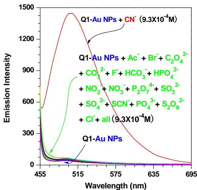
**Fig. S4** Fluorescence Emission spectra of **Q1**-Au NPs in C<sub>2</sub>H<sub>5</sub>OH in the presence of different anions(9.3×10<sup>-4</sup> mol/L). The concentration of **Q1** was 2.0×10<sup>-6</sup> mol/L and Au NPs was 6.76×10<sup>-5</sup> mol/L. Excitation wavelength (nm): 431.
