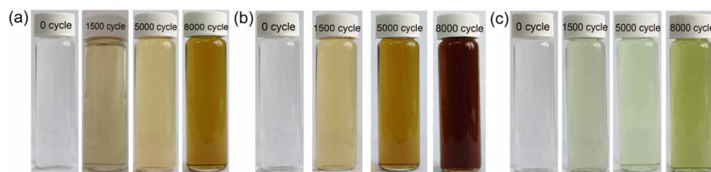
Fig. S4 The color changes of EMIMBF 4 /acetonitrile electrolyte before and after cycling at different operating temperatures: (a) -20 °C, (b) 20 °C and (c) 60 °C.
