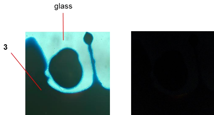
Figure S5. Optical microscopy images of an amorphous film of 3 , which was cooled from the melt under ambient conditions and stored at room temperature for 20 days. The same section (750 x 750 \mu\text{m} ) was imaged without polarizer (left) and between crossed-polarizers (right).
