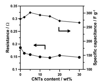
**Fig. S2.** Variation of resistance and specific capacitance of the CNTs/aMP composites with the CNT content. The resistance values were measured for a symmetric two-electrode cell using electrochemical impedance analysis at 1 kHz. The specific capacitance was estimated using integration of full cyclic voltammograms within -1 to 1 V at a scan rate of 5 mV s $^{-1}$ .
