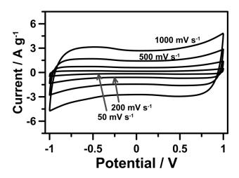
**Fig. S1.** Cyclic voltammograms of a symmetric two-electrode capacitor assembled with CNTs electrodes and 2 M  $H_2SO_4$  as the electrolyte solution. The electrodes consisted of a 1 cm<sup>2</sup> carbon film (2 mg) and a titanium foil current collector.
