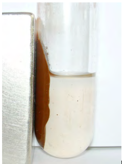
Fig. S3 Photograph of isolating Fe 3 O 4 @mSiO 2 -NHC(1) after reaction by employing an external field.
