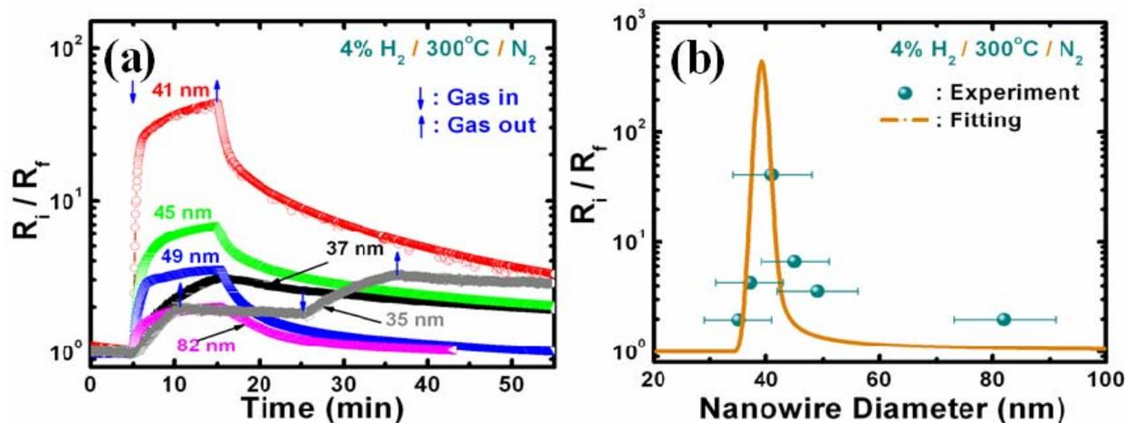
**Figure S2.** Summary of sensing properties measured at 300 °C for H<sub>2</sub> molecules diluted in N<sub>2</sub> to examine the size effect of the WO<sub>3</sub> nanowires. (a) Response of the sensors to 4% H<sub>2</sub> gas diluted in N<sub>2</sub>. (b) is the summary of (a) with a fitted curve. The fitting parameters are  $N_D = 1.1 \times 10^{18} \text{ cm}^{-3}$ ,  $\alpha = 2 \times 10^4$ ,  $V_s = 0.2 \text{ V}$ .
