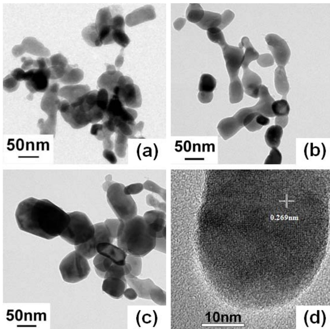
**Figure S1.** TEM micrographs of WO<sub>3</sub> nanowires for different W sputter deposition times: (a) 10 s, (b) 20 s, and (c) 60 s. (d) High-resolution TEM micrographs showing a single crystalline grain (of (a)).
