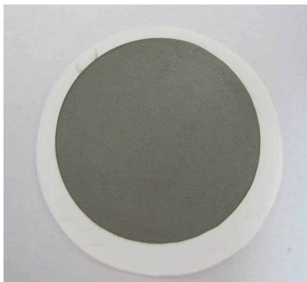
Figure S5. Digital image of freestanding films of Bi 2 Te 3 nanosheets by filtration using porous polyvinylidene fluoride (PVDF) membranes with 0.45 μm nominal pore size.
