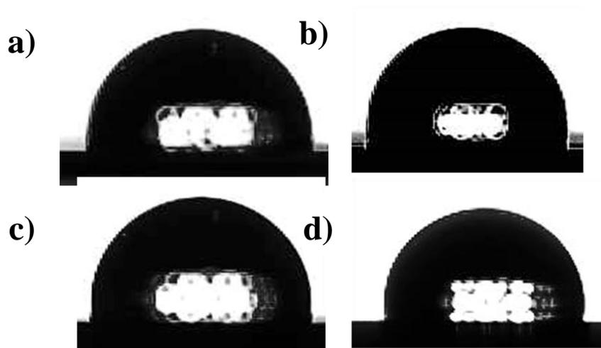
**Fig. S1.** Contact angles of various polymer electrets: a) PS, b) P(St-Fl), c) P(St-Fl)<sub>2</sub>
