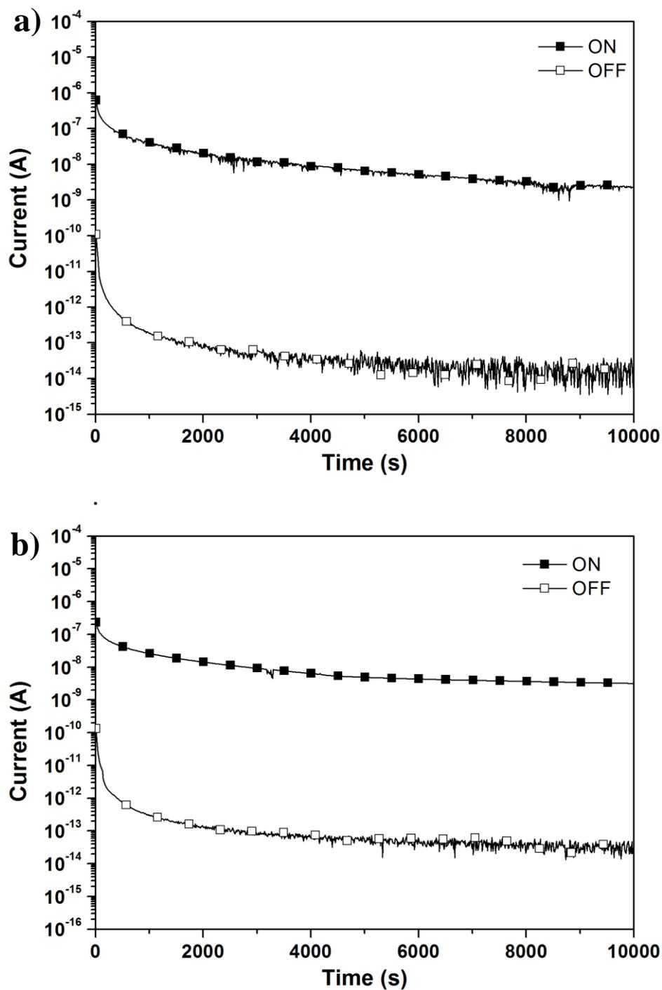
**Fig. S5.** Retention time of pentacene-based OFET memory device with a) P(St-Fl)<sub>2</sub>
