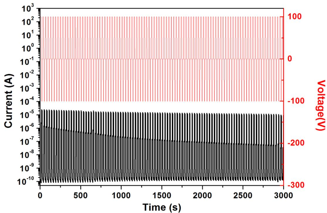
**Fig. S6.** Reversible switching for the ON- and OFF- states of pentacene-based OFET
