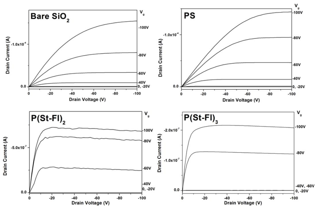
**Fig. S4.** Output characteristics of pentacene-based OFET memory devices.
