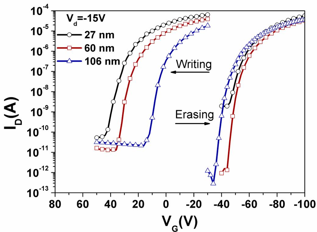
**Fig. S8.** Transfer curves of the pentacene-based OFET memory device based on the P(St-FI) polymer electret using different thicknesses.
