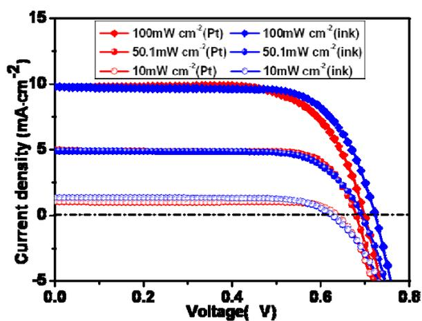
**Fig. S4** *J-V* curves of CF/ink CE-based FDSSCs ( $D_{\text{ink/CF}}$ ) and Pt wire CE-based FDSSCs ( $D_{\text{Pt wire}}$ ) with  $\text{I}_3^-/\text{I}^-$  electrolyte under different light intensities.
