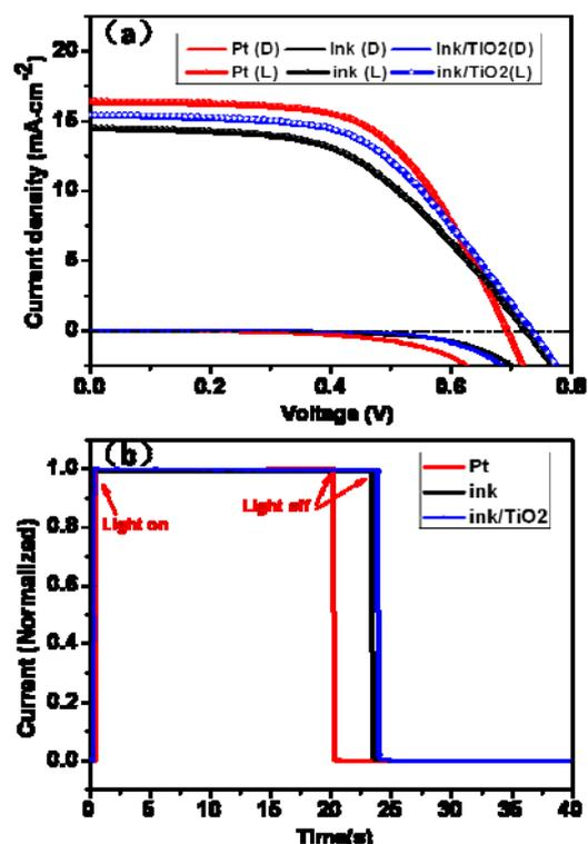
**Fig. S1** (a) *J-V* characteristics of FTO/Pt, FTO/ink and FTO/ink-TiO<sub>2</sub> CE-based PDSSCs under dark condition and standard illumination (AM 1.5G, 100mW cm<sup>-2</sup>). (b) Normalized short-circuit current-time response of FTO/Pt, FTO/ink and FTO/ink-TiO<sub>2</sub> CE-based PDSSCs during 40s.
