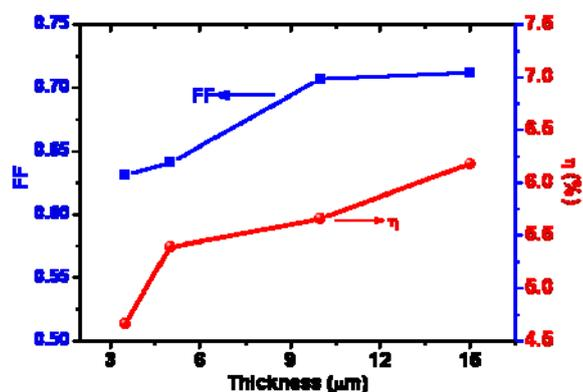
**Fig. S2** The change of fill factor (FF) and  $\eta$  of SS/ink CE-based FDSSCs as the thickness of ink film varied.
