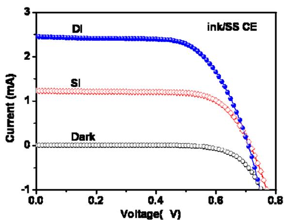
**Fig. S3** *J-V* characteristics of FDSSCs based on stainless steel (SS) wire/ink counter electrode (CE). Dark: without irradiation. SI: single-sided irradiation with  $100\text{mW cm}^{-2}$  light intensity. DI : double-sided irradiation mode with a diffuse reflector at the bottom of the device.
