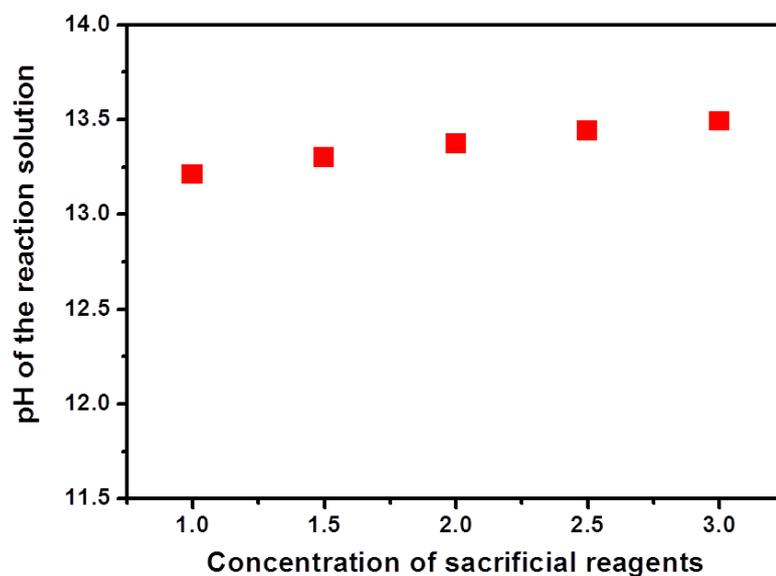
**Fig. 2S** Influence of the concentration of sacrificial reagents on the pH of the reaction solution. The abscissa denotes the multiple of used sacrificial reagent concentration compared to 0.25 M  $\text{Na}_2\text{SO}_3$ /0.35 M  $\text{Na}_2\text{S}$ . For example, when the abscissa was 2.0, 0.50 M  $\text{Na}_2\text{SO}_3$ /0.70 M  $\text{Na}_2\text{S}$  were used.
