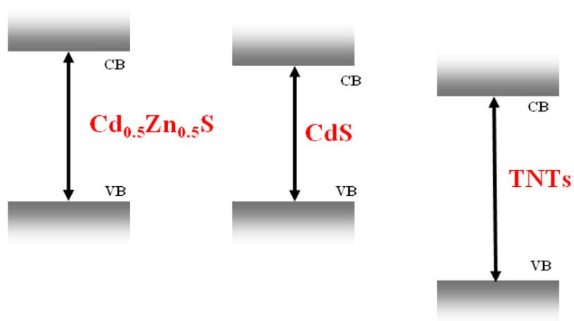
**Fig. 1S** Schematic diagram of the band positions of  $\text{Cd}_{0.5}\text{Zn}_{0.5}\text{S}$ ,  $\text{CdS}$  and  $\text{TNTs}$ .
