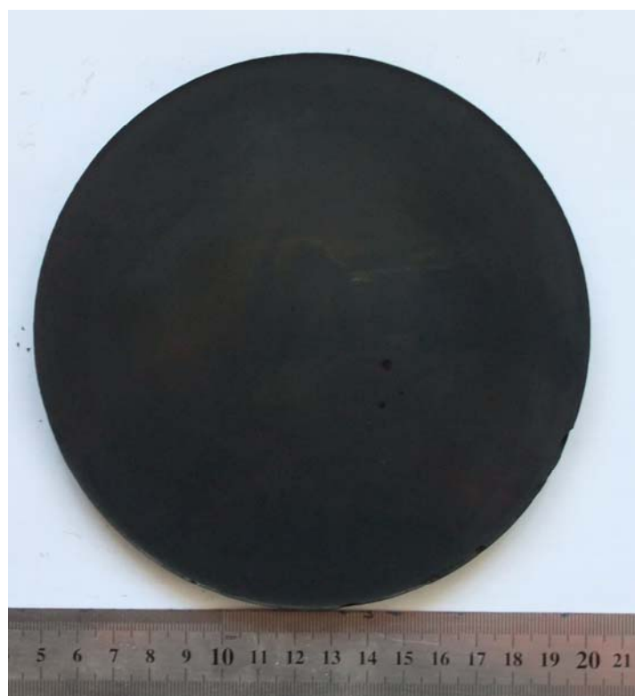
Figure S3. Typical large-sized SiOC aerogel-like monolith produced from a mixture of PSO and PDMS (20 cSt/85 wt %), (pyrolysis temperature: 1000 °C).
