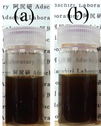
**Figure S1.** Photographs of magnetite nanoparticles synthesized at 300 °C: (a) Dispersed in water solution; (b) Dispersed in 0.9% NaCl solution
