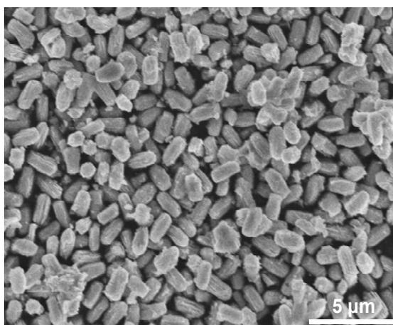
**Figure S1** SEM image for porous Ga<sub>2</sub>O<sub>3</sub> particles with a low magnification mode, showing the uniformity of the particle sizes and their morphology.
