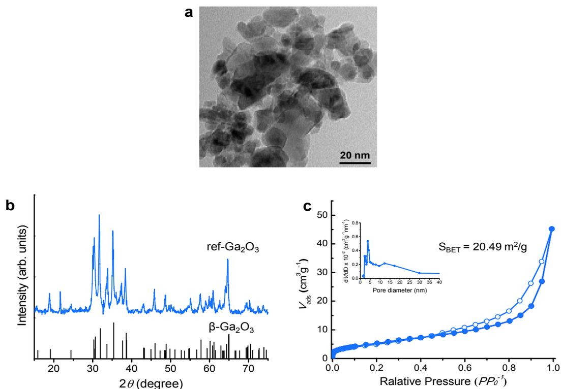
**Figure S3** (a) TEM image, (b) XRD pattern, and (c) nitrogen adsorption-desorption isotherm where the pore size distribution of the ref-Ga<sub>2</sub>O<sub>3</sub> is shown as its inset.
