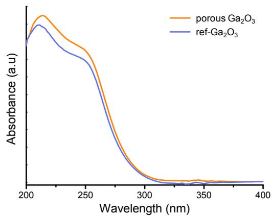
**Figure S4** The UV-vis diffuse spectra of porous Ga<sub>2</sub>O<sub>3</sub> and ref-Ga<sub>2</sub>O<sub>3</sub> samples. The solid state UV-vis diffuse reflectance spectra were recorded using a JASCO V-570 spectrometer. The absorption edge of both samples is approximately 280nm.
