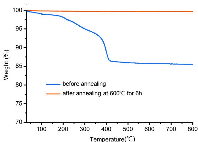
**Figure S2** Thermal gravimetric analysis of porous Ga<sub>2</sub>O<sub>3</sub> particles before and after annealing at 600°C for 6 hours.
