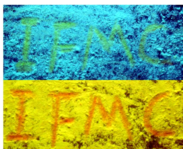
**Fig. S15** The samples **1A** (up) and **2A** (down) were cast on the filter paper and the letters "IFMC" were written with a spatula under UV-light at room temperature.
