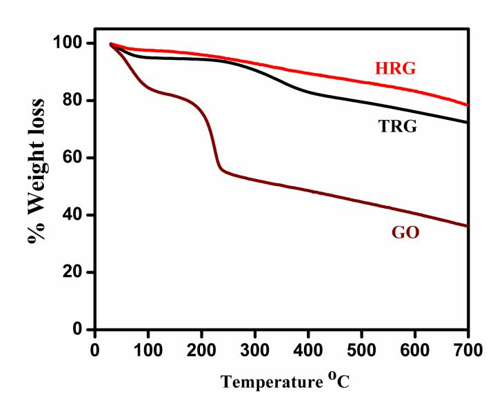
Figure 1 Thermogravimetric analysis (TGA) plot for graphite oxide (GO), trigol reduced graphene (TRG) and hydrazine reduced graphene (HRG)
