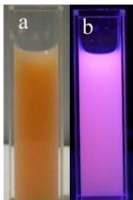
Fig. S5 Images of the fNPs emulsion illuminated by a) sunlight; b) 365 nm of UV light.
