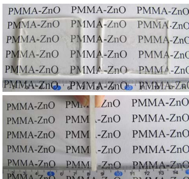
Figure S1. Photos of 4 cm (diameter) × 0.4 cm (thickness) PMMA/ZnO-1 and -2 sheets. The refractive index is about 1.4444 for both PMMA/ZnO-1 and -2.
