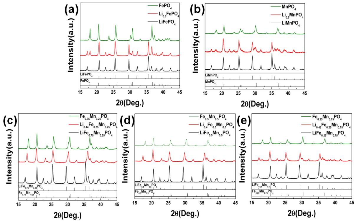
**Figure S4** (a) Evolution of XRD patterns of (a)  $\text{Li}_{1-y}\text{FePO}_4$  (b)  $\text{Li}_{1-y}\text{MnPO}_4$ , (c)  $\text{Li}_{1-y}\text{Fe}_{0.75}\text{Mn}_{0.25}\text{PO}_4$ , (d)  $\text{Li}_{1-y}\text{Fe}_{0.5}\text{Mn}_{0.5}\text{PO}_4$ , and (e)  $\text{Li}_{1-y}\text{Fe}_{0.25}\text{Mn}_{0.75}\text{PO}_4$  [ $0 \leq y \leq 1$ ] with a delithiation process.
