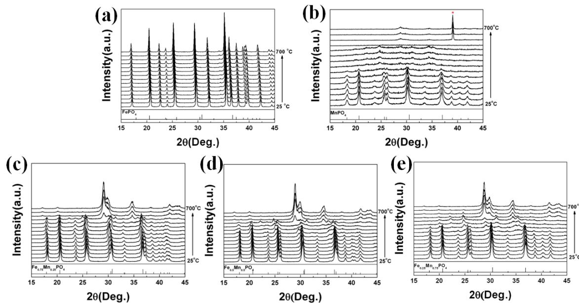
**Figure S5** *in-situ* XRD patterns of fully delithiated (a)  $\text{FePO}_4$ , (b)  $\text{MnPO}_4$  (\* : the XRD peak of Pt holder), (c)  $\text{Fe}_{0.75}\text{Mn}_{0.25}\text{PO}_4$ , (d)  $\text{Fe}_{0.5}\text{Mn}_{0.25}\text{PO}_4$ , and (e)  $\text{Fe}_{0.25}\text{Mn}_{0.75}\text{PO}_4$  at temperature from 25°C to 700°C and at  $2\theta$  from 15° to 45°
