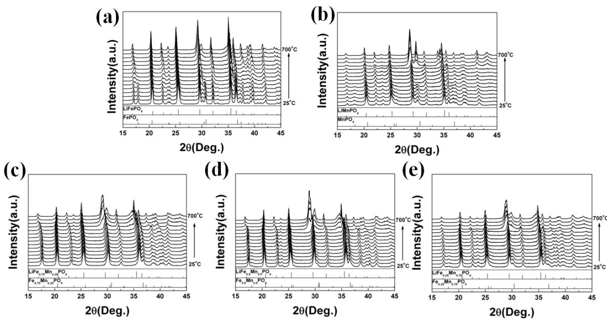
**Figure S6** *in-situ* XRD patterns of partially delithiated (a)  $\text{Li}_{0.6}\text{FePO}_4$ , (b)  $\text{Li}_{0.5}\text{MnPO}_4$ , (c)  $\text{Li}_{0.44}\text{Fe}_{0.75}\text{Mn}_{0.25}\text{PO}_4$ , (d)  $\text{Li}_{0.4}\text{Fe}_{0.5}\text{Mn}_{0.25}\text{PO}_4$ , and (e)  $\text{Li}_{0.46}\text{Fe}_{0.25}\text{Mn}_{0.75}\text{PO}_4$  at temperature from 25°C to 700°C and at  $2\theta$  from 15° to 45°
