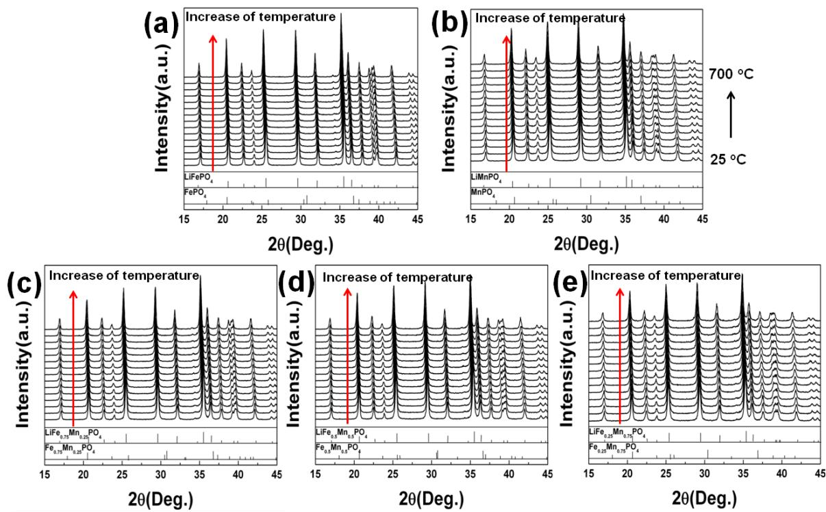
**Figure S2** *in-situ* XRD patterns of as-prepared (a)  $\text{LiFePO}_4$ , (b)  $\text{LiMnPO}_4$ , (c)  $\text{LiFe}_{0.75}\text{Mn}_{0.25}\text{PO}_4$ , (d)  $\text{LiFe}_{0.5}\text{Mn}_{0.5}\text{PO}_4$ , and (e)  $\text{LiFe}_{0.25}\text{Mn}_{0.75}\text{PO}_4$  at temperature from 25°C to 700°C and at 2θ from 15° to 45°
