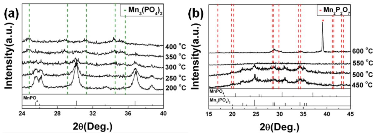
**Figure S8** (a) *in-situ* XRD patterns of fully delithiated MnPO<sub>4</sub> at temperature from 200°C to 400°C and at 2θ from 24° to 40° and (b) *in-situ* XRD patterns of fully delithiated MnPO<sub>4</sub> at temperature from 450°C to 600°C and at 2θ from 15° to 45° (\* : the XRD peak of Pt holder)
