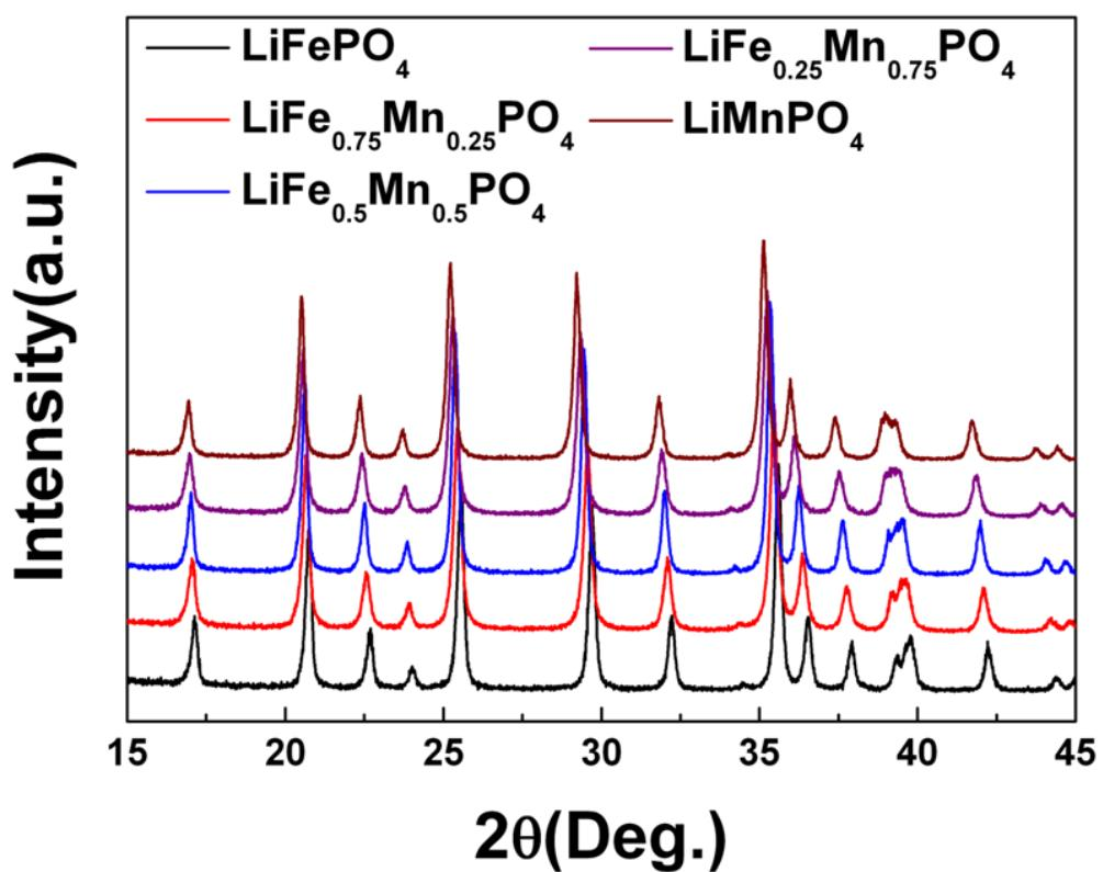
**Figure S1** XRD patterns of as-prepared  $\text{LiFe}_{1-x}\text{Mn}_x\text{PO}_4$  [ $0 \leq x \leq 1$ ]
