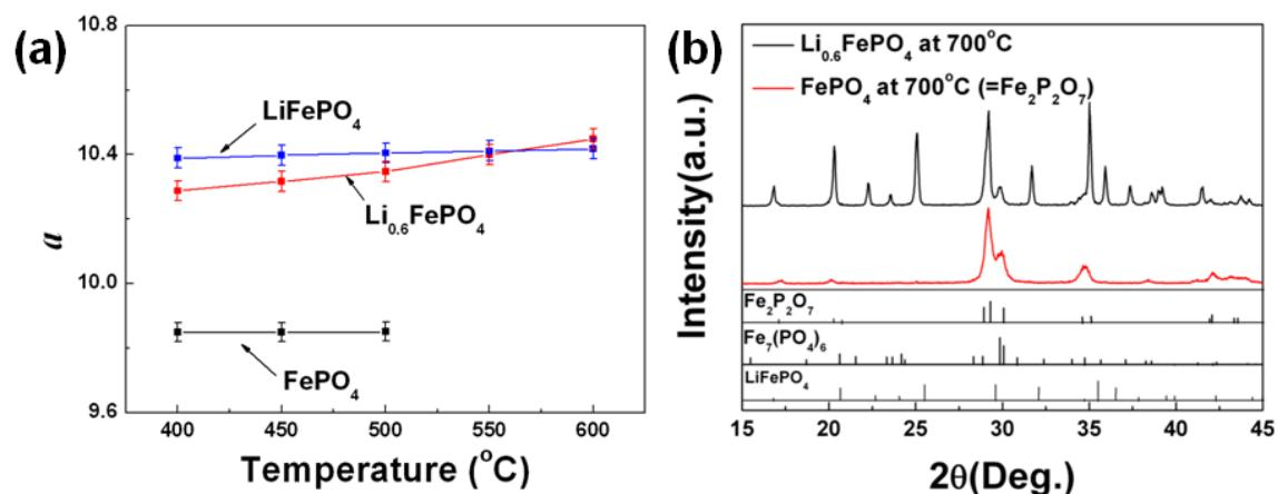
**Figure S7** (a) Comparison of lattice parameter  $a$  of  $\text{Li}_y\text{FePO}_4$  [ $y = 0$ ,  $0.6$ , and  $1$ ] varied by temperature and (b) XRD patterns of partially delithiated  $\text{Li}_{0.6}\text{FePO}_4$  at  $700^{\circ}\text{C}$  compared with  $\text{Fe}_2\text{P}_2\text{O}_7$  and  $\text{Fe}_7(\text{PO}_4)_6$  among at  $2\theta$  from  $15^{\circ}$  to  $45^{\circ}$ .
