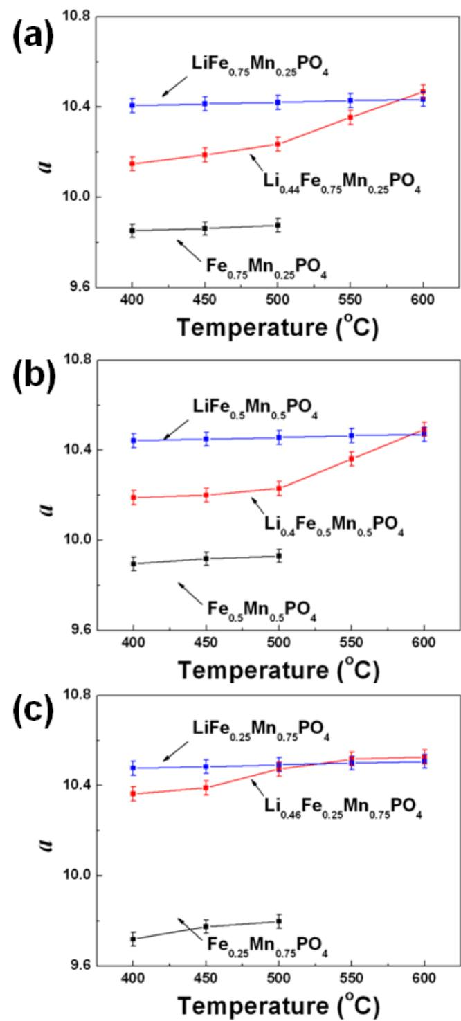
**Figure S9** Comparison of lattice parameter  $a$  of (a)  $\text{Li}_y\text{Fe}_{0.75}\text{Mn}_{0.25}\text{PO}_4$  [ $y = 0, 0.44, 1$ ], (b)  $\text{Li}_y\text{Fe}_{0.5}\text{Mn}_{0.5}\text{PO}_4$  [ $y = 0, 0.4, 1$ ], and (c)  $\text{Li}_y\text{Fe}_{0.25}\text{Mn}_{0.75}\text{PO}_4$  [ $y = 0, 0.46, 1$ ] varied by temperature
