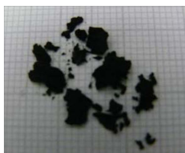
Figure S2 Carbon flakes as prepared (1 square = 1 mm 2 )
