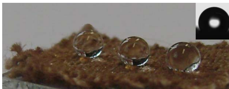
Figure S4. Water droplet standing on the textile coated with \text{Fe}_3\text{O}_4 .
