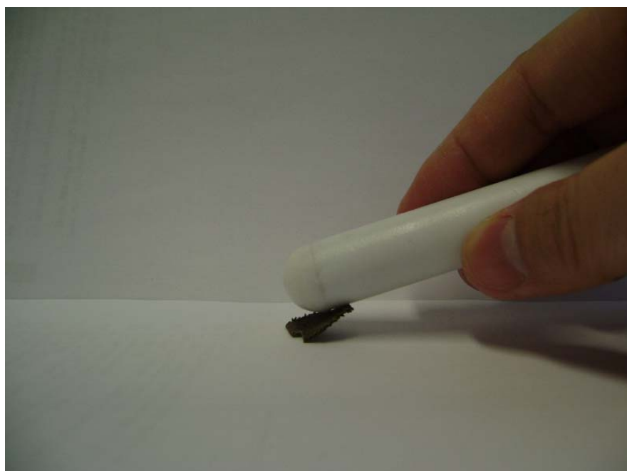
Figure S6. A photo showing that the textile coated with \text{Fe}_3\text{O}_4 is magnetic when a magnet is close to it.
