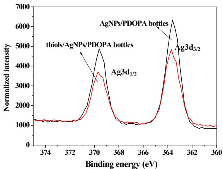
**Fig. S5** Ag3d spectra of AgNPs/PDOPA (LBL three times) SPE bottle and thiol/AgNPs/PDOPA SPE bottle.
