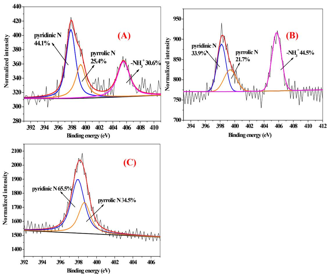
**Fig. S4** Peak fitting of N1s spectra of (A) three layers of PDOPA films coated SPE bottle, (B) thiols/PDOPA coated (LBL three times) SPE bottle, and (C) AgNPs/PDOPA coated (LBL three times) SPE bottle.
