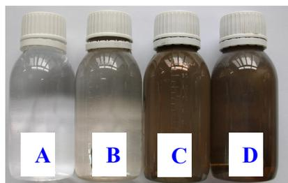
**Fig. S1** Images of (A) bare PET bottle, (B) PDOPA film coated PET bottle, (C) AgNPs/PDOPA PET bottle, and (D) thiols/AgNPs/PDOPA bottles.
