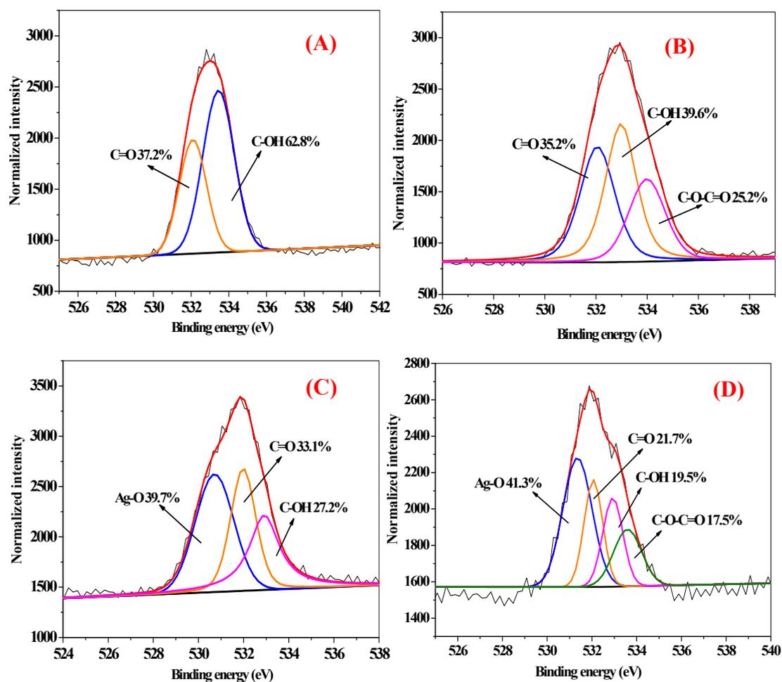
**Fig. S3** Peak fitting of O1s spectra of (A) three layers of PDOPA films coated SPE bottle, (B) thiols/PDOPA coated (LBL three times) SPE bottle, (C) AgNPs/PDOPA coated (LBL three times) SPE bottle, and (D) thiols/AgNPs/PDOPA coated SPE bottle (LBL three times).
