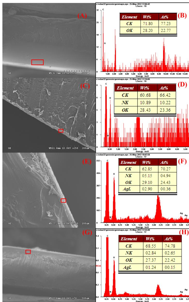
**Fig. S6** SEM images of cross-section of (A) PET bottle, (C) one layer of PDOPA film coated bottles, (E) AgNPs/PDOPA coated (LBL one time) bottles, and (G) AgNPs/PDOPA coated (LBL twice) bottles; (B), (D), (F), (H) the corresponding EDX mapping and element composition of the marked section in each bottle sample.
