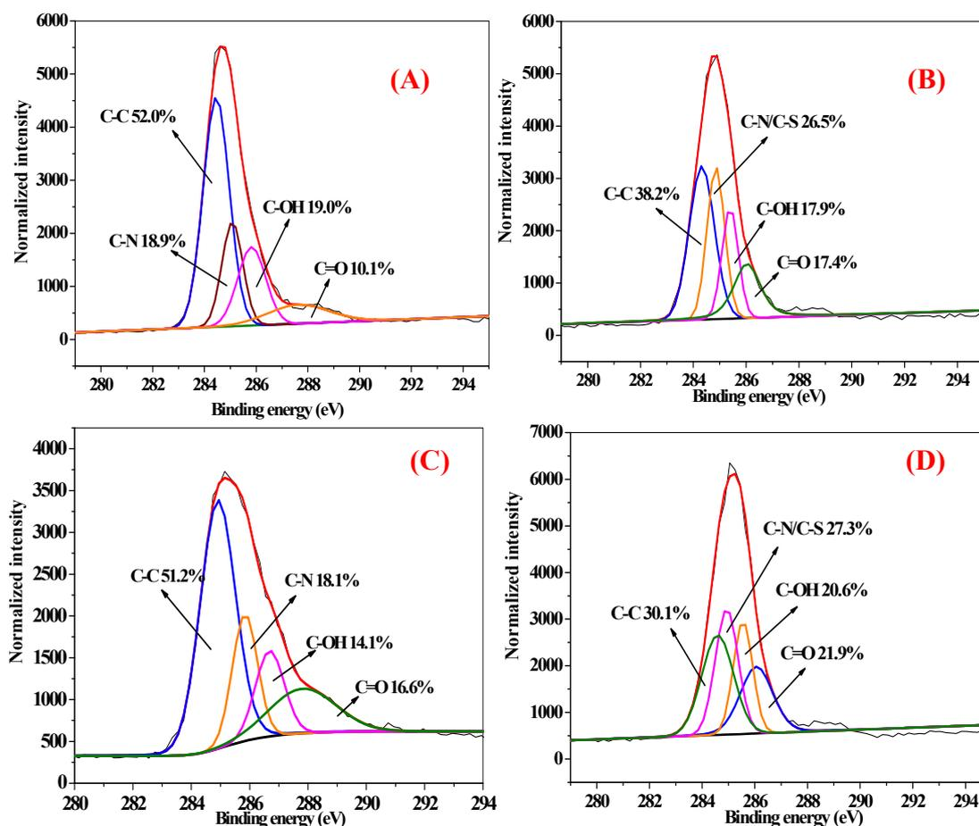
**Fig. S2** Peak fitting of C1s spectra of (A) three layers of PDOPA films coated SPE bottle, (B) thiols/PDOPA coated (LBL three times) SPE bottle, (C) AgNPs/PDOPA coated (LBL three times) SPE bottle, and (D) thiols/AgNPs/PDOPA coated SPE bottle (LBL three times).
