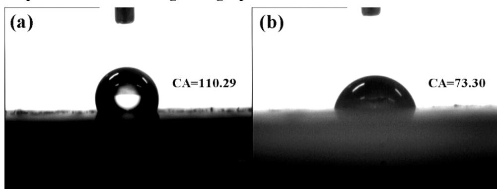
Fig.S3 The equilibrium contact angles of graphite (a) and GA-G (b)
