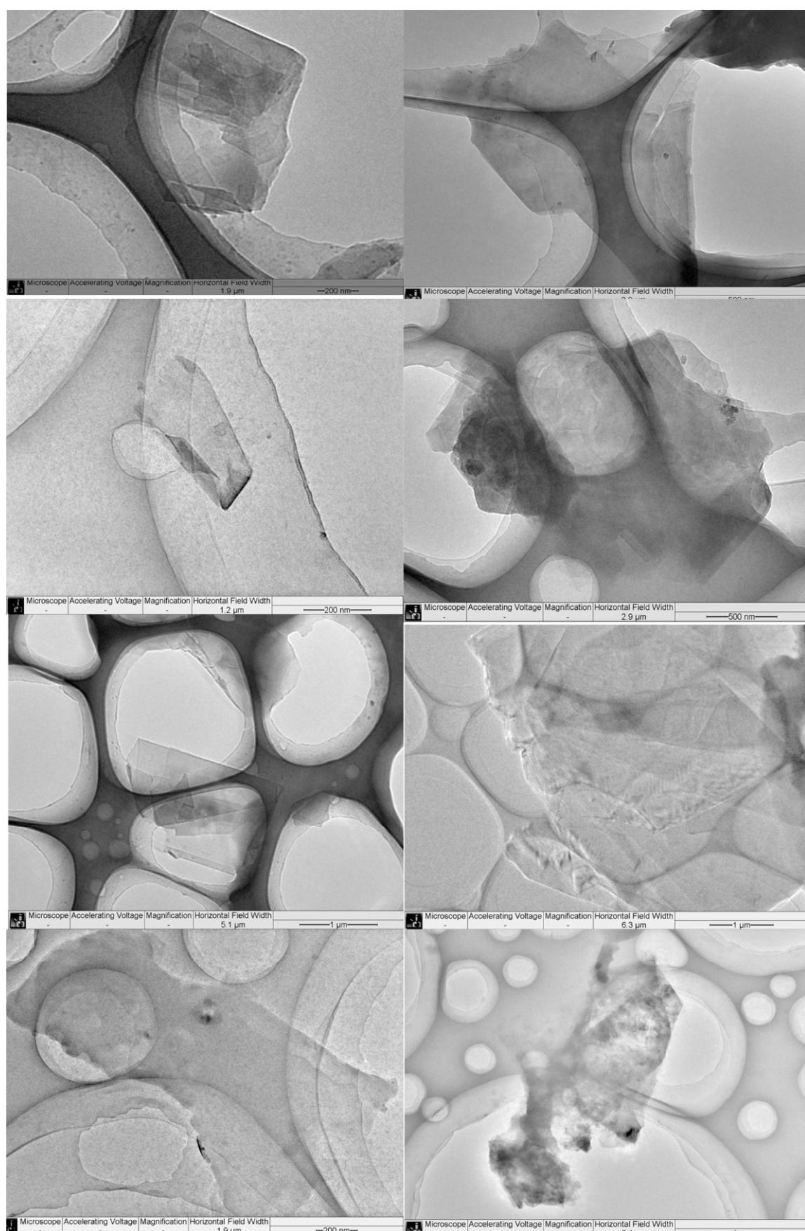
Fig.S1 Low magnification TEM images of folded and stacked GA-G nanosheets
